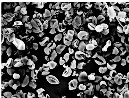
Figure 1.8 SEM of a microcapsule encapsulating polyethylene imine catalyst.
