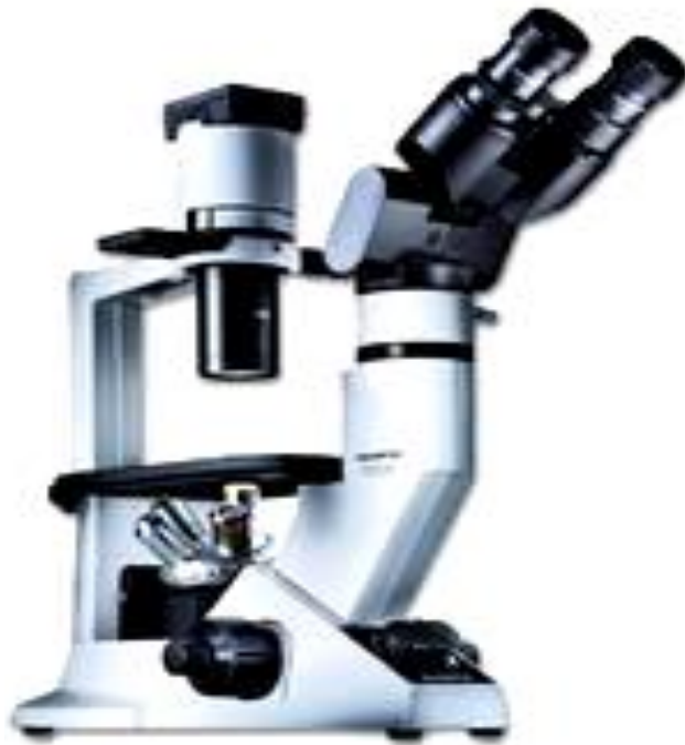
Figure 5. Inverted microscope (Olympus® Hamburg, Germany) used throughout this study for monitoring germination of Fusarium and Trichoderma conidia.
