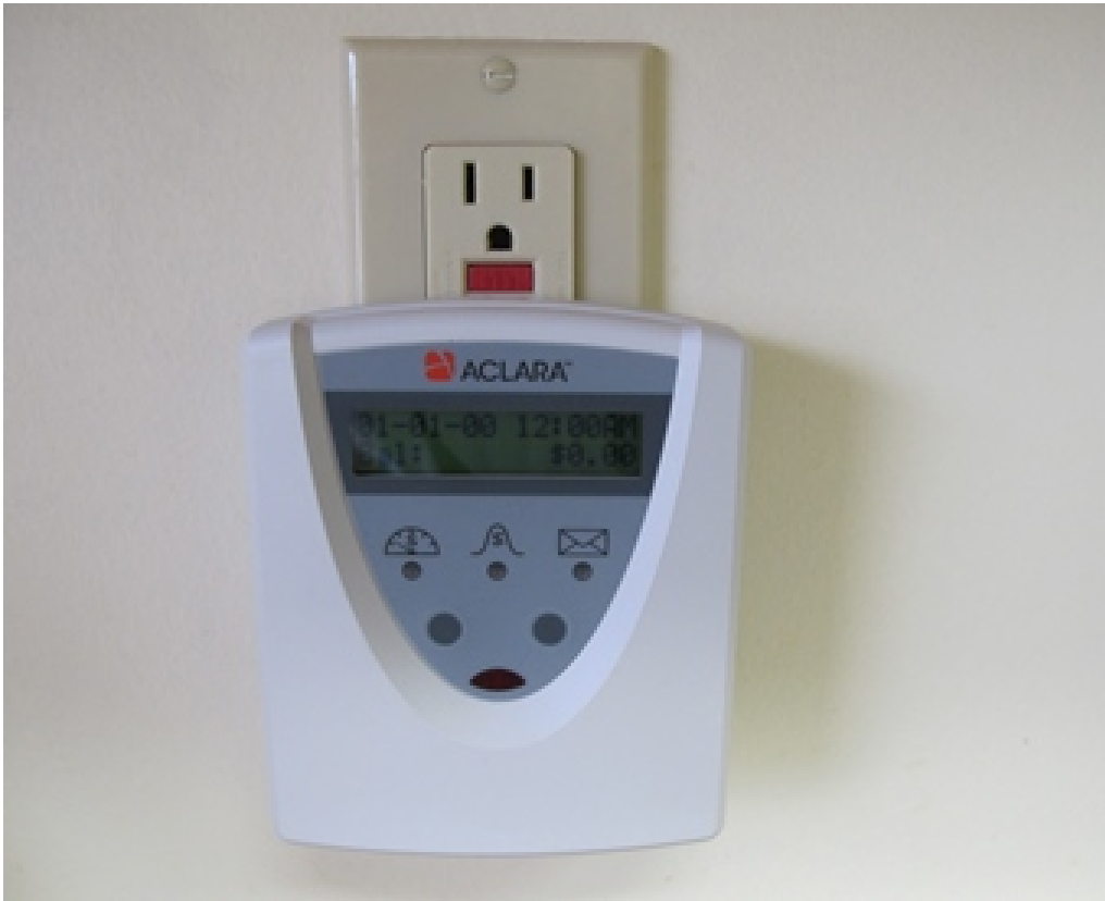
Figure 2.3 In-Home Display (IHD) Used by Jackson Electric
