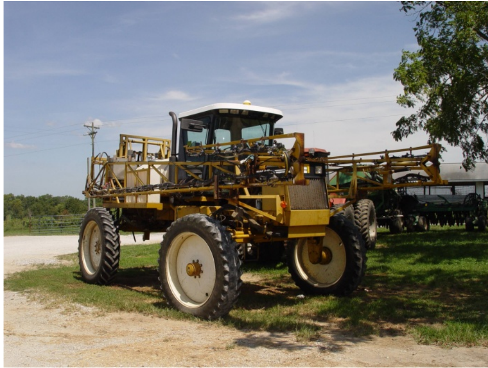
Figure 2.1: RoGator 664 self-propelled sprayer with 24 m boom and map-based single nozzle control system.
