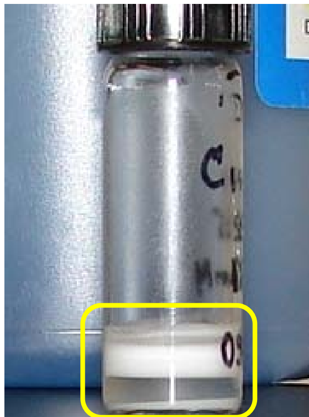
Figure 6.6. Photograph of a sample that was subjected to the “vortexing procedure”. Three distinct fractions of silica C18 particles in SDS solution are clearly distinguishable. Image was adapted from [163].
