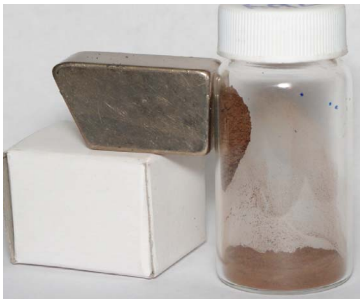
Figure 3.4. Photograph showing the magnetic properties of the iron oxide/zeolite composites
