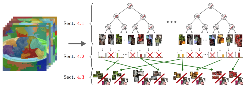
Figure 2.1: Discriminative component mining using Random Forest. For each superpixel, the LAB color feature and SURF feature are encoded by Fisher Vector. Random Forest is used to hierarchically cluster the feature vectors of superpixels of the training images. The discriminative clusters in the leaves are selected and used to train the component model. [7]
