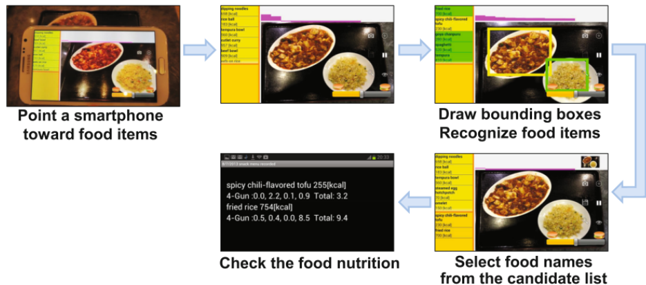
Figure 2.3: FoodCam system process flow. Users draw bounding boxes over each food item and image classification is performed for each bounding box region. Top-5 candidate food items are displayed on the screen for users to choose from.
