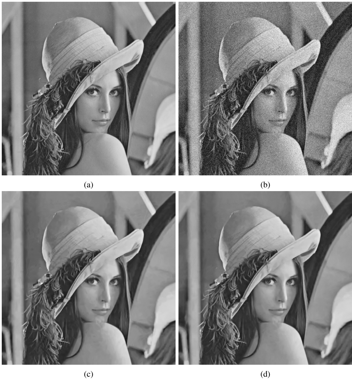
Figure 5.8: Subjective Comparison of Lena Image (a) Original Lena Image. (b) AWGN added with \sigma = 20 (c) Denoised Image using BM3D (PSNR=33.05) (d) Denoised Image using Proposed Method (PSNR=34.46)
