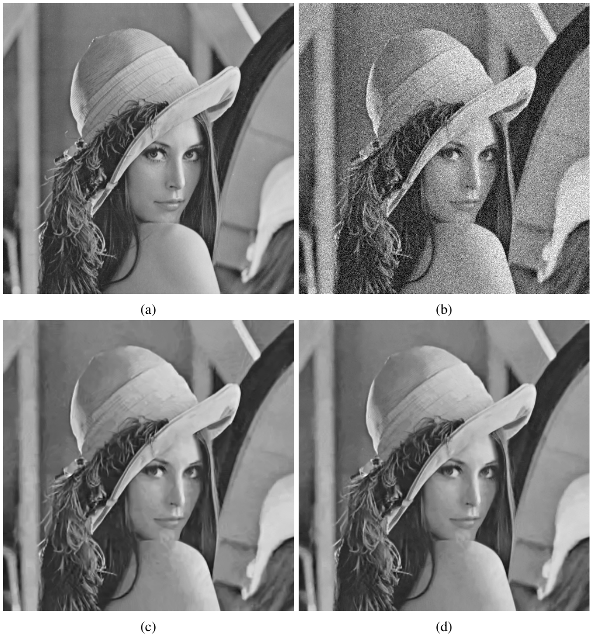
Figure 5.9: Subjective Comparison of Lena Image (a) Original Lena Image. (b) AWGN added with \sigma = 30 (c) Denoised Image using BM3D (PSNR=31.26) (d) Denoised Image using Proposed Method (PSNR=32.78)
