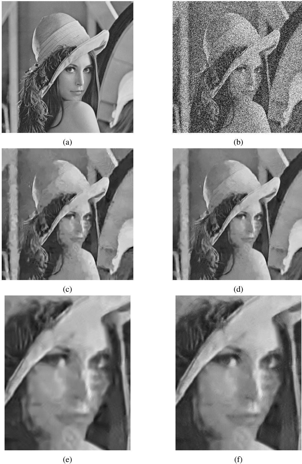
Figure 5.5: Subjective Comparison of Lena Image (a) Original Lena Image. (b) AWGN added with \sigma = 100 (c) Denoised Image using BM3D (d) Denoised Image using Proposed Method (e) Face Cropped from BM3D Output (f) Face cropped from Proposed Method Output
