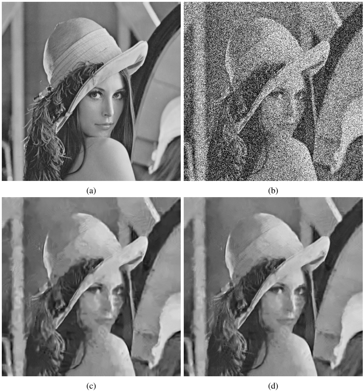
Figure 5.16: Subjective Comparison of Lena Image (a) Original Lena Image. (b) AWGN added with \sigma = 100 (c) Denoised Image using BM3D (PSNR=25.95) (d) Denoised Image using Proposed Method (PSNR=27.54)
