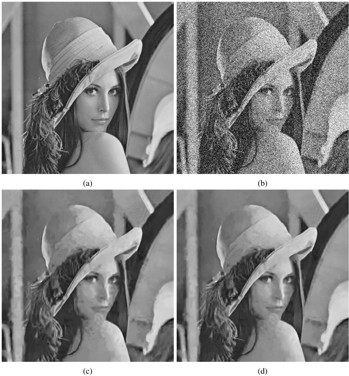
Figure 5.13: Subjective Comparison of Lena Image (a) Original Lena Image. (b) AWGN added with \sigma = 70 (c) Denoised Image using BM3D (PSNR=27.57) (d) Denoised Image using Proposed Method (PSNR=29.10)
