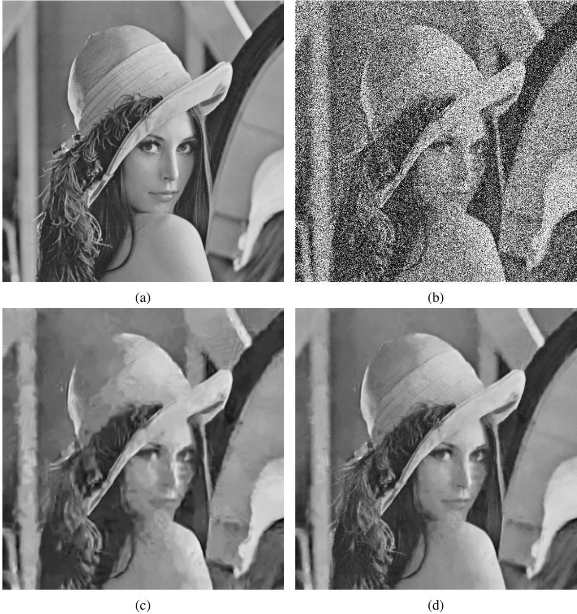
Figure 4.4: Performance of Denoised Image (a) Original Lena image (b) Noise image with \sigma = 100 (c) Original BM3D Algorithm (PSNR = 25.95) (d) Best BM3D Image (PSNR = 29.21)
