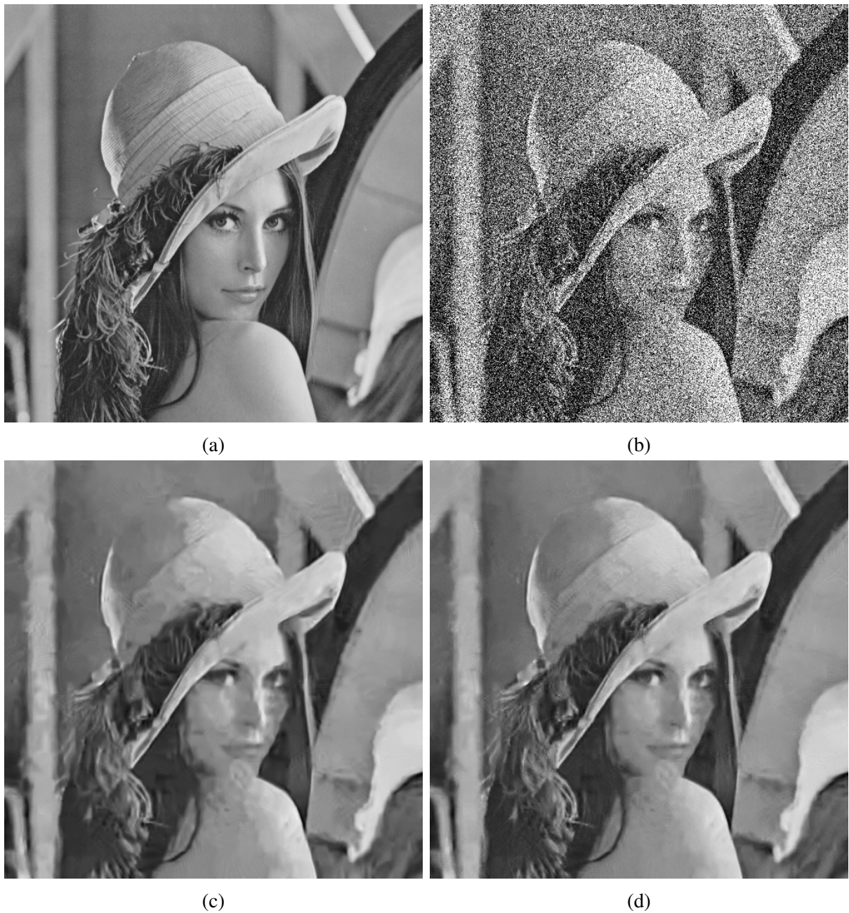
Figure 5.14: Subjective Comparison of Lena Image (a) Original Lena Image. (b) AWGN added with \sigma = 80 (c) Denoised Image using BM3D (PSNR=26.97) (d) Denoised Image using Proposed Method (PSNR=28.53)
