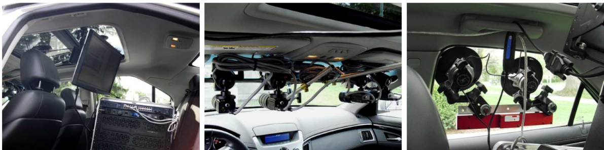
Figure 3.1: The RoadLab in-vehicle laboratory: a) (left): on-board computer and LCD screen, b) (center): dual stereo front visual sensors, c) (right): side stereo visual sensors [4].
