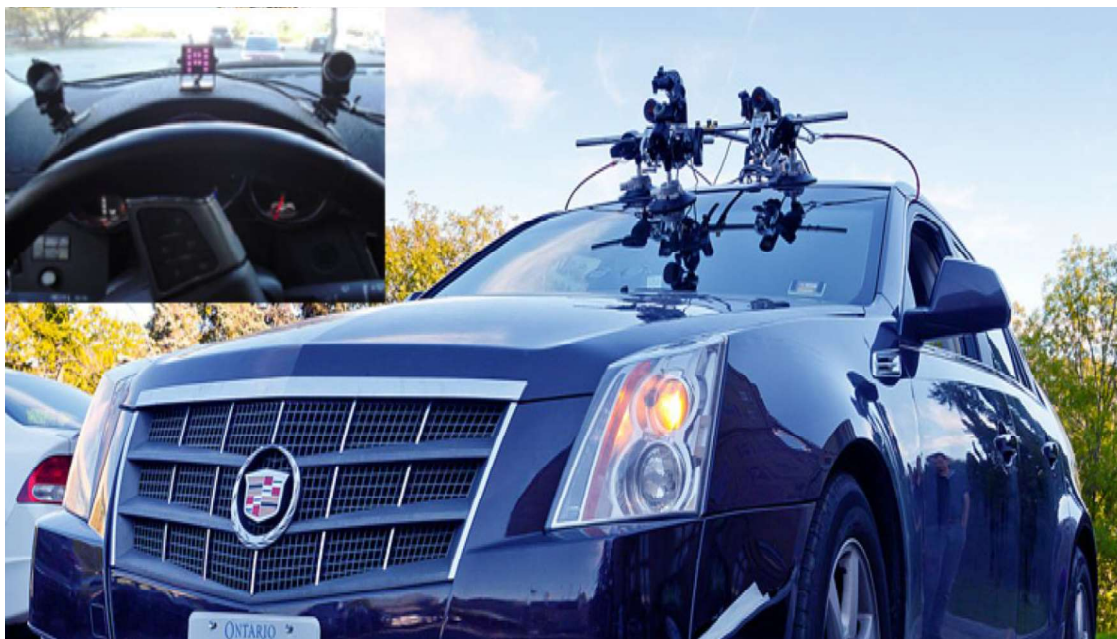
Figure 3-1. Equipped car used in RoadLAB to provide Driver-Environment-Vehicle data stream.
