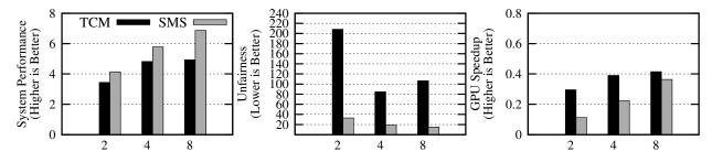
Figure 5.8. SMS vs TCM on a 16 CPU/1 GPU system with varying the number of channels
