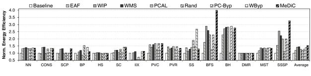
Figure 4.12. Energy efficiency of MeDiC.
