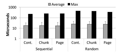
**Figure 7.3.** Demand paging load-to-use latencies measured on NVIDIA GTX 1080 for sequential and random access patterns using contiguous, chunked, page-granularity allocation. Y axis is in log scale. Error bars represent one standard deviation of variance.
