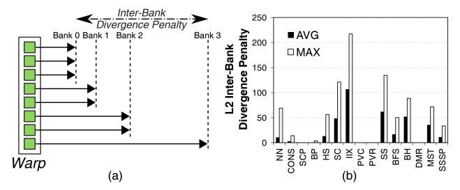
**Figure 4.7.** Effect of bank queuing latency divergence in the L2 cache: (a) example of the impact on stall time of skewed queuing latencies, (b) inter-bank divergence penalty due to skewed queuing for all-hit warps, in cycles.
