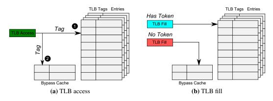
Figure 6.14. TLB fill bypassing logic in MASK.
