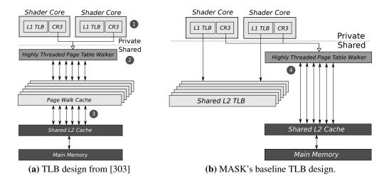
**Figure 6.2.** Baseline TLB designs. (a) shows the baseline proposed by [303]. (b) shows the baseline used in this dissertation.
