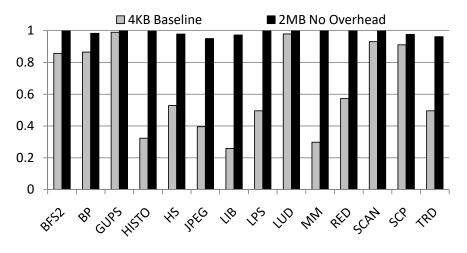
**Figure 7.2.** Comparison of performance between two memory protection designs: a multi-level TLB with 4KB pages and an optimized multi-level TLB with 2MB pages.
