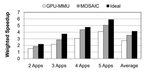
**Figure 7.9.** Heterogeneous workload performance with a different number of concurrent applications.
