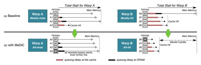
**Figure 4.5.** (a) Existing inter-warp heterogeneity, (b) exploiting the heterogeneity with MeDiC to improve performance.
