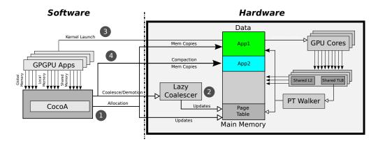
**Figure 7.7.** The overall design of Mosaic. (1) **CONTIGUITY-CONSERVING ALLOCATION** provides the soft-guarantee allowing LAZY-COALESCER to coalesce pages transparently. (2) coalesce requests are sent to LAZY-COALESCER prior to kernel launch (3). (4) **CONTIGUITY-AWARE COMPACTION** provides physical space contiguity and reduces the amount of fragmentation.
