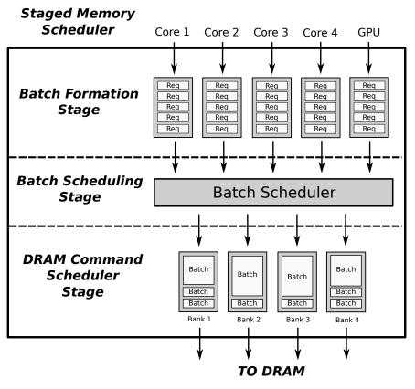
Figure 5.4. The design of SMS
