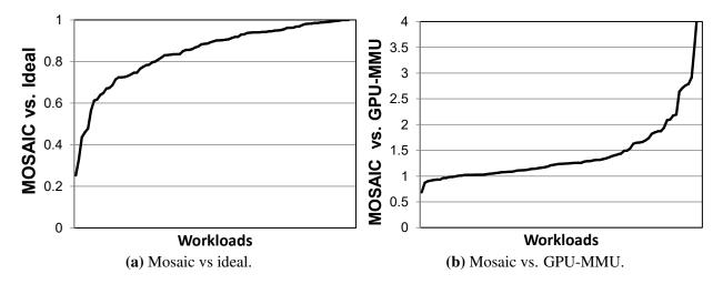
**Figure 7.12.** The performance of Mosaic across 235 workloads. (a) shows the performance of Mosaic relative to the ideal performance with no address translation overhead. (b) shows the performance of Mosaic relative to previously proposed state-of-the-art TLB design [303]
