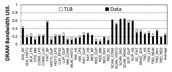
Figure 6.10. Bandwidth breakdown of two applications.
