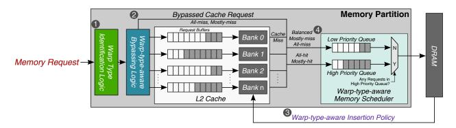
Figure 4.10. Overview of MeDiC: 1 warp type identification logic, 2 warp-type-aware cache bypassing, 3 warp-type-aware cache insertion policy, 4 warp-type-aware memory scheduler.
