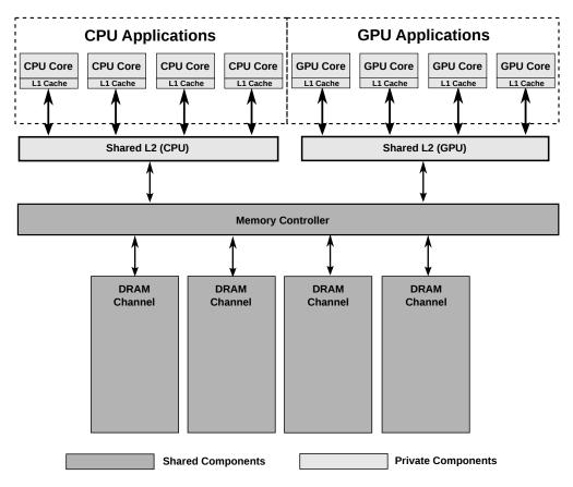
Figure 2.3. The memory hierarchy of a heterogeneous CPU-GPU architecture.
