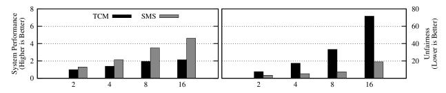
Figure 5.7. SMS vs TCM on a 16 CPU/1 GPU, 4 memory controller system with varying the number of cores
