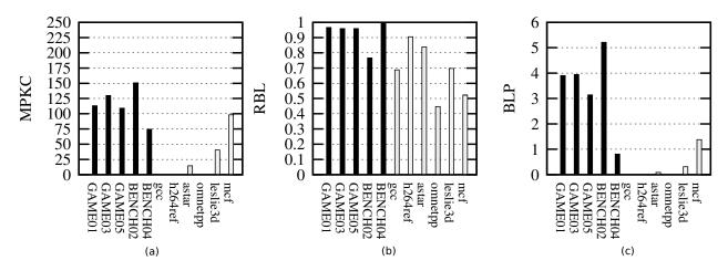
**Figure 5.2.** GPU memory characteristic. (a) Memory-intensity, measured by memory requests per thousand cycles, (b) Row buffer locality, measured by the fraction of accesses that hit in the row buffer, and (c) Bank-level parallelism.
