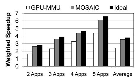
**Figure 7.8.** Homogeneous workload performance with a different number of concurrent applications.
