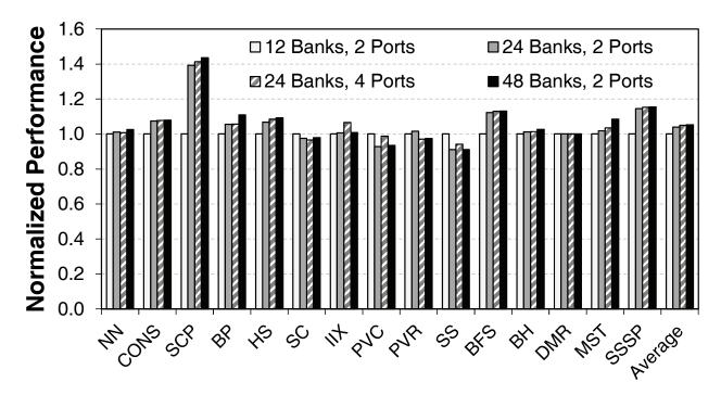
**Figure 4.9.** Performance of GPGPU applications with different number of banks and ports per bank, normalized to a 12-bank cache with 2 ports per bank.
