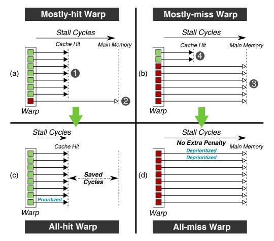
**Figure 4.1.** Memory divergence within a warp. (a) and (b) show the heterogeneity between *mostly*-*hit* and *mostly-miss* warps, respectively. (c) and (d) show the change in stall time from converting *mostly-hit warps into all-hit warps*, and *mostly-miss warps into all-miss warps*, respectively.
