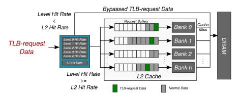
Figure 6.15. The design of TLB-REQUEST-AWARE L2 BYPASS.
