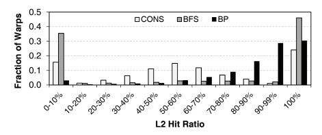
**Figure 4.3.** L2 cache hit ratio of different warps in three representative GPGPU applications (see Section 4.4 for methods).
