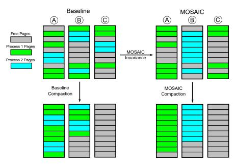
**Figure 7.6.** The difference between the baseline compaction mechanism and CAC showing that CAC always preserve soft-guarantee imposed by **COCOA**.
