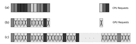
**Figure 5.1.** Limited visibility example. (a) CPU-only information, (b) Memory controller's visibility, (c) Improved visibility
