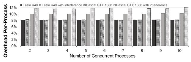
Figure 6.1. Context switch overheads under contention on K40 and GTX 1080.
