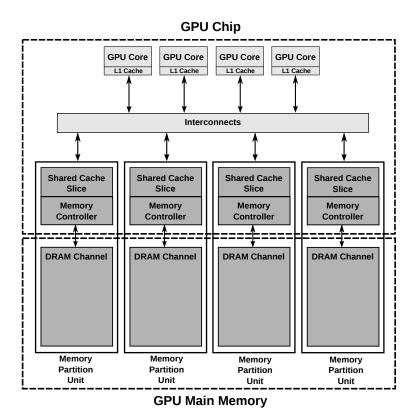
Figure 2.2. Overview of a modern GPU architecture.
