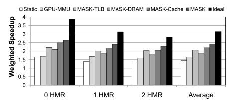
Figure 6.17. System-wide weighted speedup for multiprogrammed workloads.
