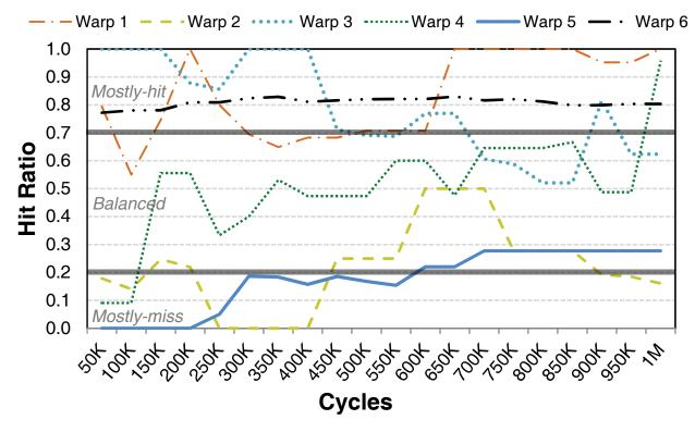
Figure 4.6. Hit ratio of randomly selected warps over time.
