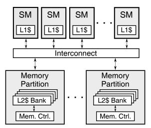
Figure 4.2. Overview of the baseline GPU architecture.
