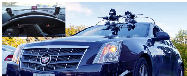
Figure 2.1: Vehicular instrumentation configuration. a) (top-left): In-vehicle non-contact infra-red binocular gaze tracking system. b): Forward scene stereo imaging system mounted on the roof of the vehicle.
