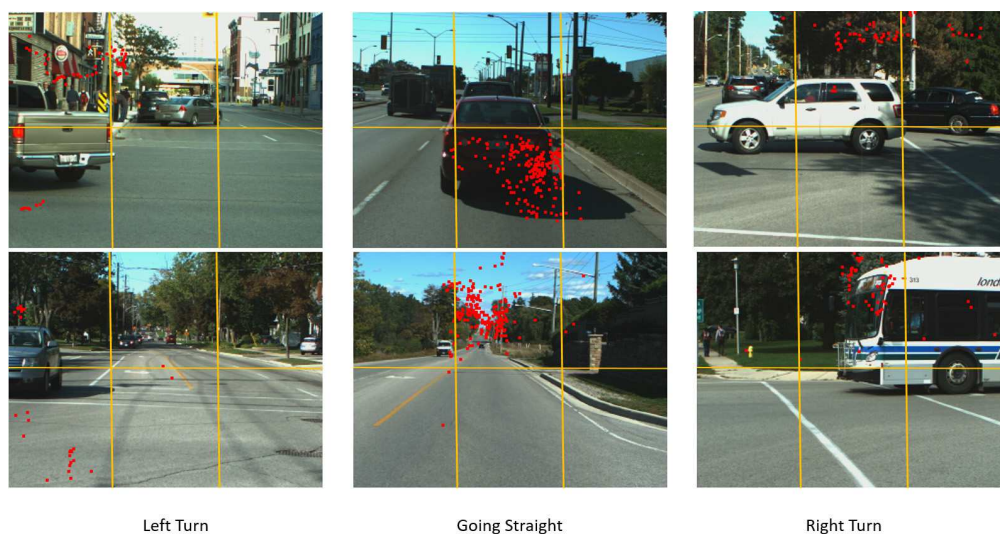
Figure 5.4: Gaze points are shown on driving images 5 seconds before a left turn, going straight, and a right turn. Images are divided into six regions.
