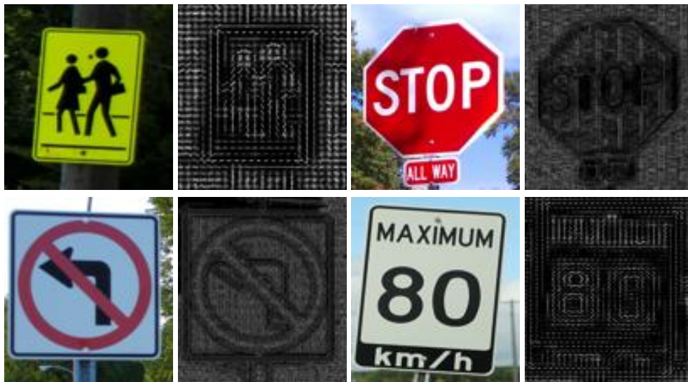
Figure 4.5: Examples of HOG features extracted from traffic signs.
