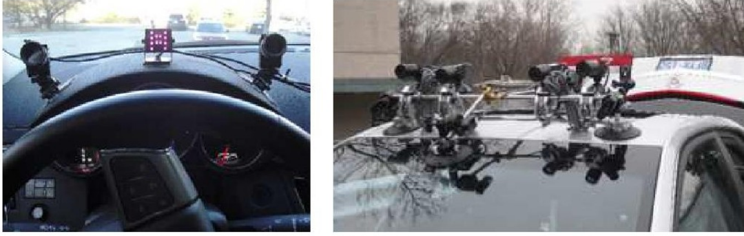
Figure 4.1: Physical configuration (left): Remote eye tracking system. (right): RoadLAB stereoscopic vision system.
