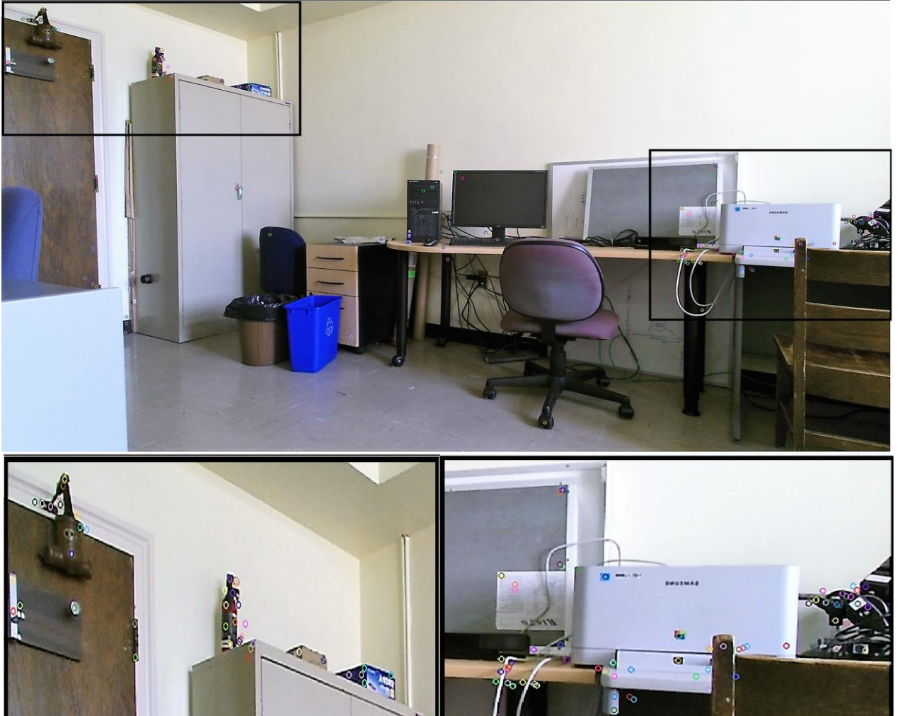
Figure 5.2 Case 1: Feature Points. The bottom images zoom in the black region of the top one. Those colorful dots are SURF feature points detected from feature detection phases.
