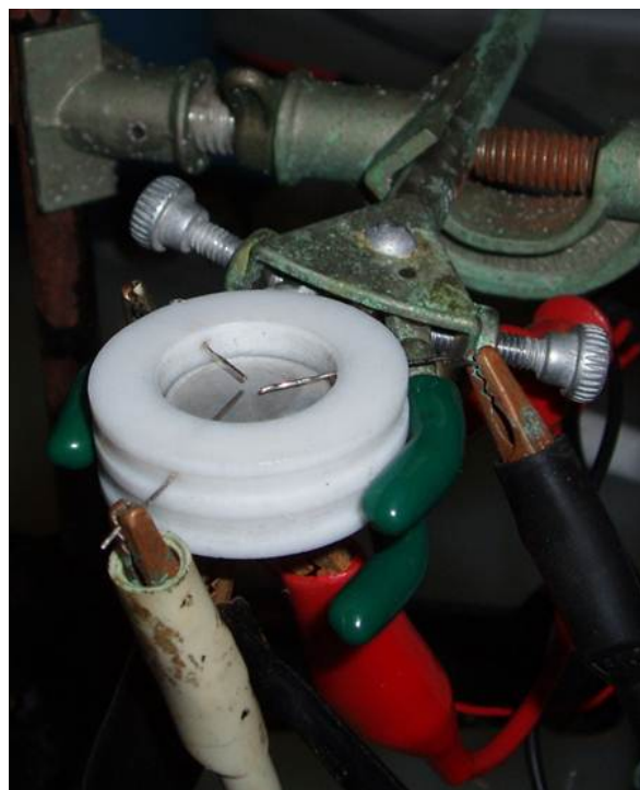
Figure 13. Photograph of the second generation sonoelectrochemical cell constructed with a Teflon sleeve to hold a thin layer of electrolyte above the transducer and around the wire electrodes. The surface of transducer is the metallic disk seen below the three electrodes that are separated by 120 degrees and pointed toward the center. All electrodes are composed of platinum wire. The transducer is not in electrical contact with the electrodes.
