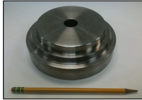
Figure 1-2. Conical mold insert to receive micro-texture.
