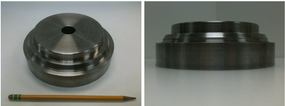
Figure 4-1. Conical mold insert considered for micro-texturing.
