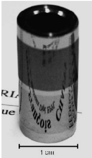
Figure 2-5 [24] . Hollow titanium cylinder covered with micro-cavities.
