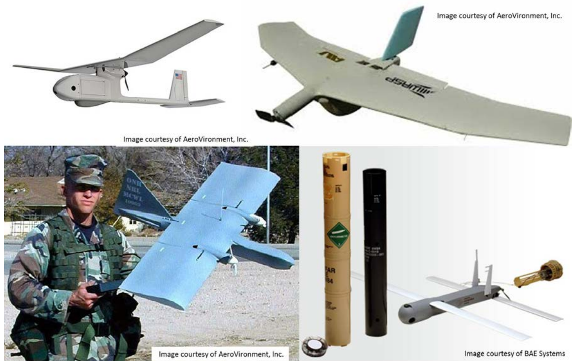
Figure 1.2 Examples of deployable UAV's top left ) Raven [6], top right ) Wasp [6], bot left ) Dragon Eye [6], bot right ) tube launched Coyote II [7]
