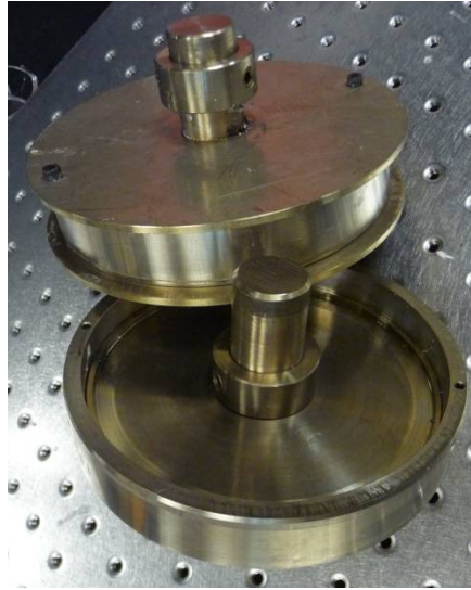
Figure 2-6 – Micropatterned cylinders. Originally designed as bearings, these cylinders with micropatterned surfaces served as the rollers for this machine.
