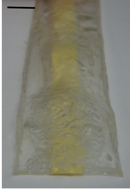
Figure 2-12 – Hazards of embedding improper materials. Embedding materials that can retain humidity, such as the paper demonstrated here, causes major defects as the heat of the process causes the water to vaporize while the PDMS is curing. Scale bar shown in the upper left is equal to 12 mm (~0.5”).
