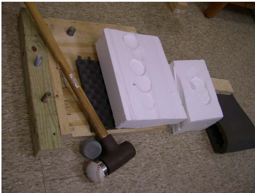
Figure 4.19 Surfaces Tested in Lab Impact Test
