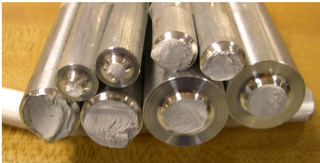
Figure 5.30 Close Up of Broken Pins
