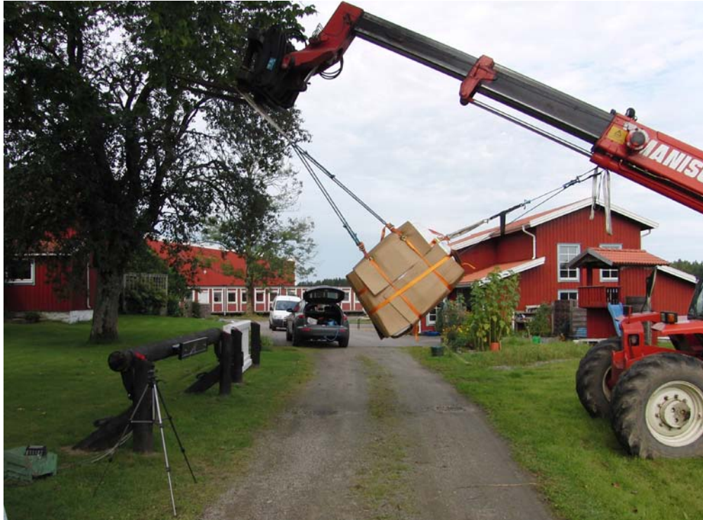
Figure 4.4 Mim Construction Pendulum Impact Test [25]
