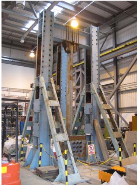
Figure 4.1 Pendulum Tester at TRL in England [53]
