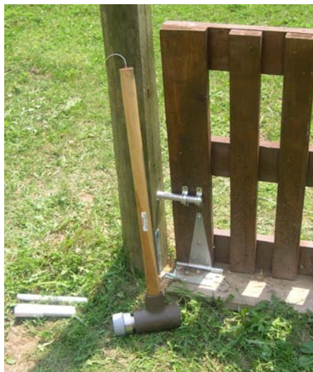
Figure 5.23 Field Testing Setup and U-bracket Constraints
