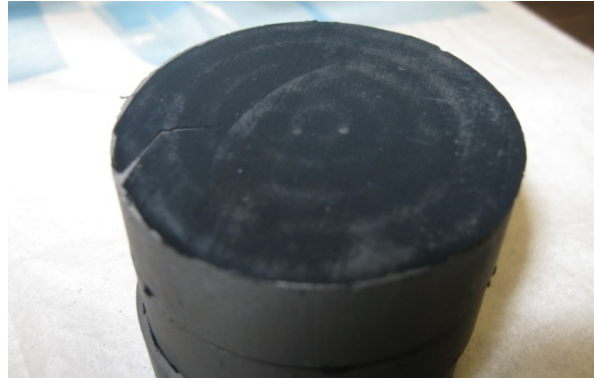
Figure 4-14 - Aligned MWCNT Array - Post Graphitization
