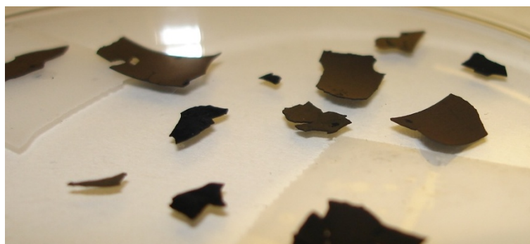
Figure 4-8 - Bronze coloration seen on MWCNT arrays after extreme O 2 plasma etching
