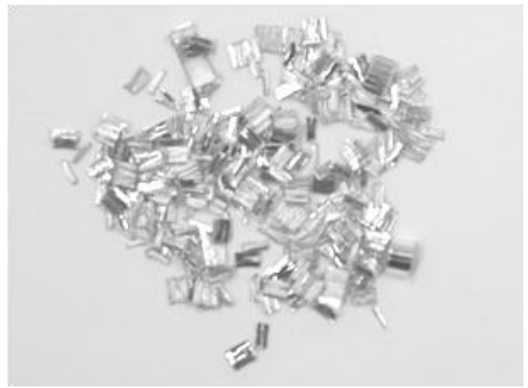
Figure 3.27: Microstructures of the machined surface and chip morphology after cryogenic machining under different cutting speeds: (a) 50 m/min; (b) 100 m/min; and (c) 150 m/min ( f = 0.25 mm/rev, r_n = 70 μm).
