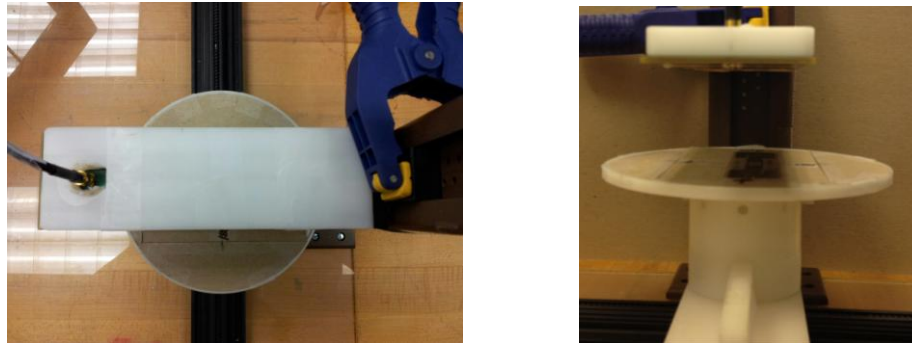
Figure 64: Static Offset test at the “0” or “no offset” position. Top view (left) and side view (right)
