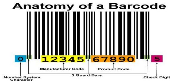
Figure 2: Anatomy of a Bar Code
