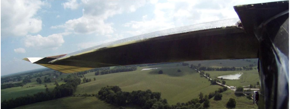
Figure 6-24: Control surfaces during left roll, note aileron deflected for right roll
