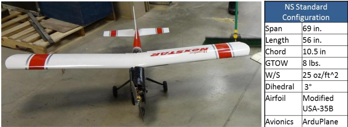
Figure 6-1: Airframe Specs for – Flight Test 1
