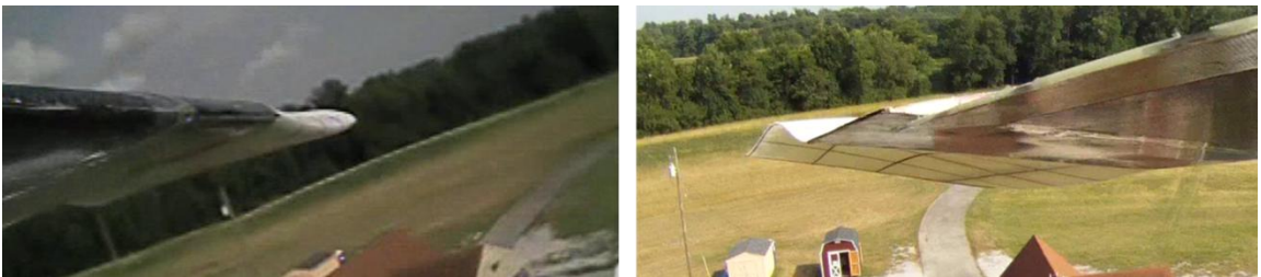
Figure 6-18: Wing shape during 1.5g pull-up at 26kts
