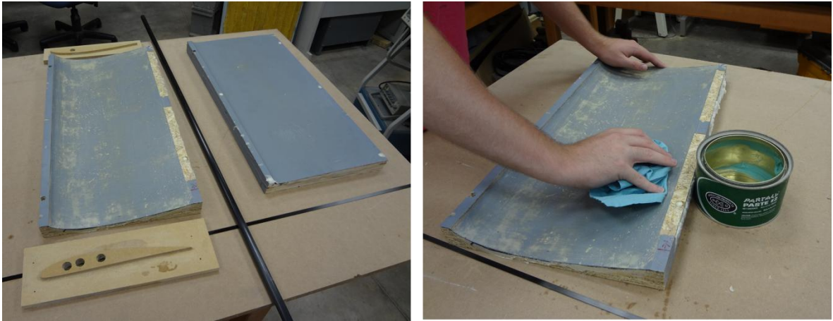
Figure 4-9: A) Four part mold and torque tube B) Mold being waxed for pour
