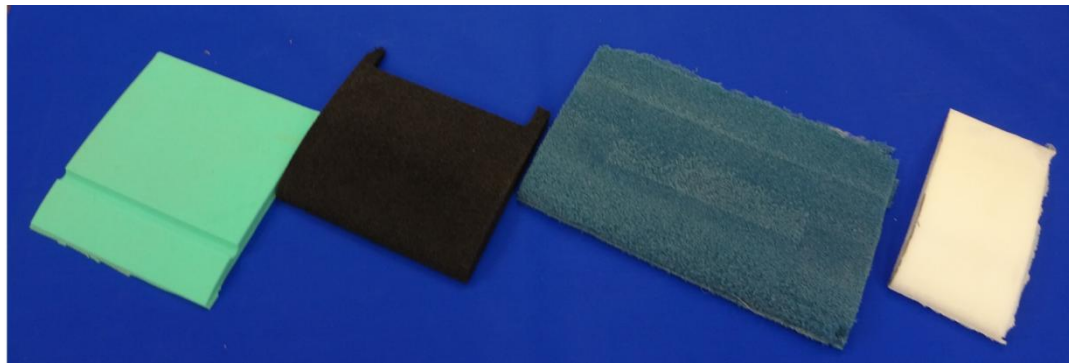
Figure 4-2: Foams tested: A) polyurethane, B) high density polyethylene, C) low density polyethylene, D) AB Foam
