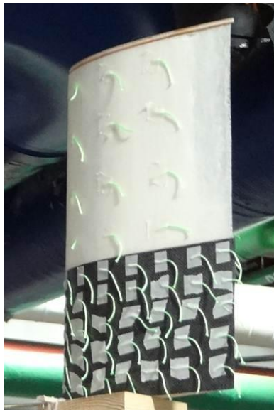
Figure 5-5: Tufts on wing to confirm flow direction
