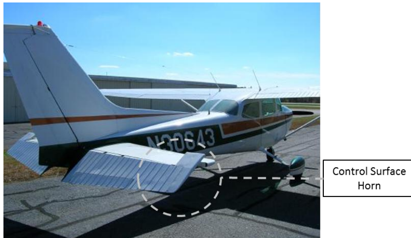
Figure 5-12: Example of a counter balanced control surfaces ( www.airmart.com )
