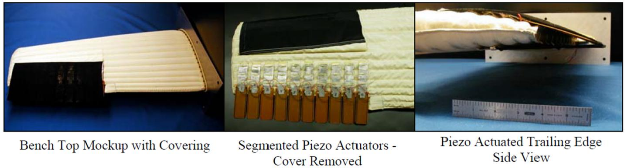
Figure 2-12: ILC Dover piezoelectric actuated trailing edge on a Vectran inflatable wing [26]
