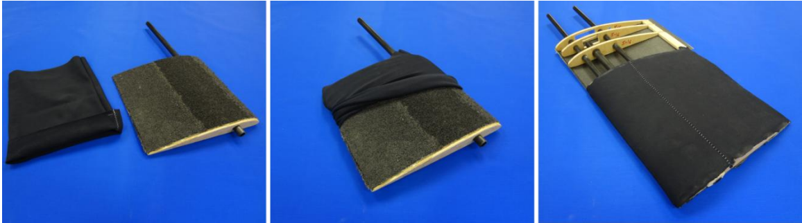
Figure 4-8: Black foam wings with fabric skinned being applied
