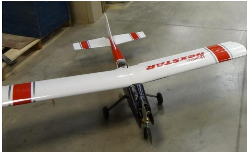
Figure 3-1: UK NexStar converted for autonomous operation
