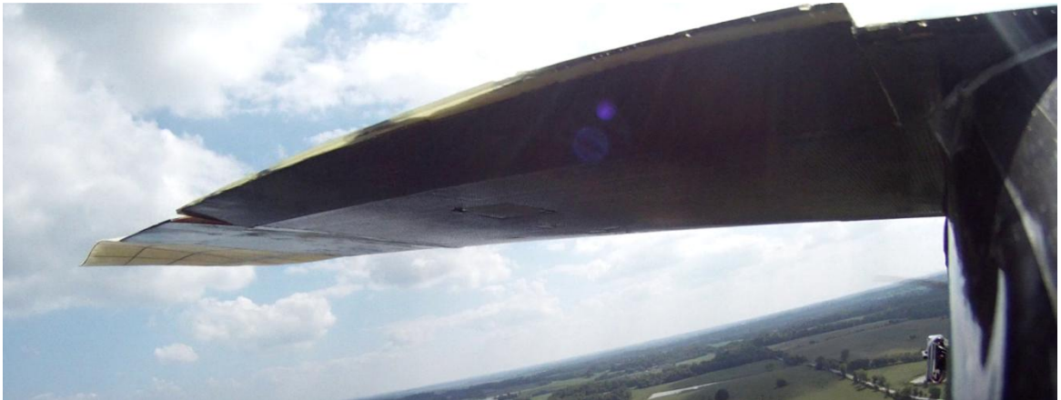
Figure 6-23: Control surfaces during right roll, note aileron deflected for left roll
