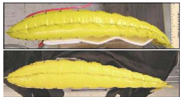
Figure 2-11: Left) Nitinol actuator for an inflatable wing-Right) Actuated and zero deflections [18]
