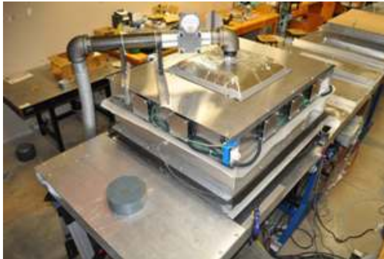
Figure 3.5: Blowing rig V.2 installed on TCFF.
