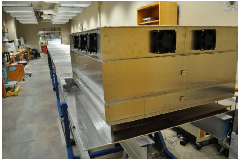
Figure 3.2: Upstream view of TCFF with blowing rig V.1 installed above test section.
