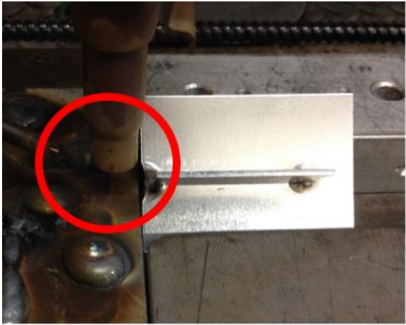
Pre-heating electrode position
