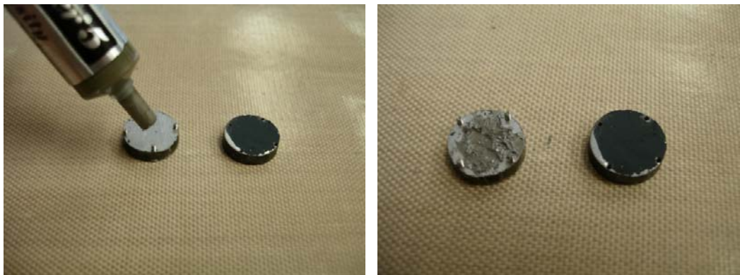
Figure 4.17 Even, homogenous coverage of Arctic Silver 5 Thermal Compound on the top aluminum substrate
