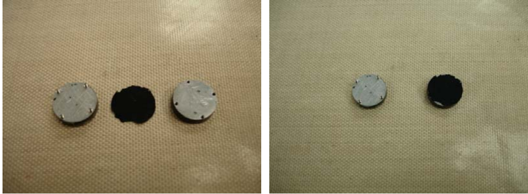
Figure 4.16 Placement of MWCNT array onto aluminum cap-screw assembly
