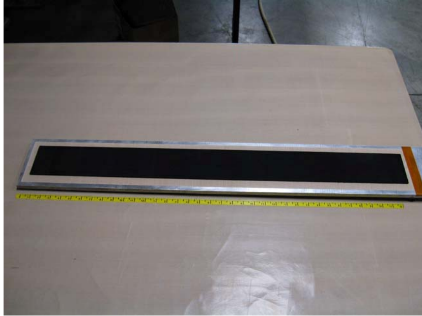
Figure 1.5 3"x36" section of MWCNT array
