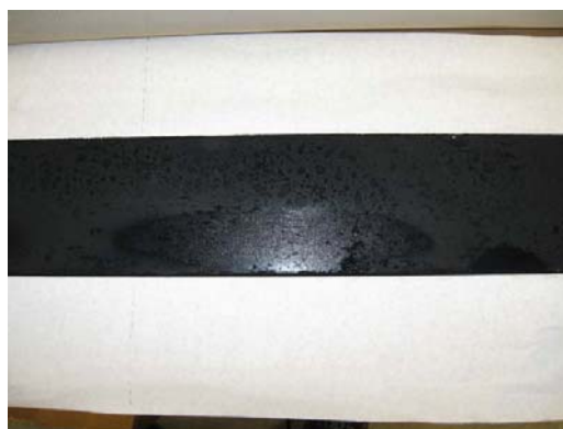
Figure 4.5 The MWCNT array drying after water cleaning
