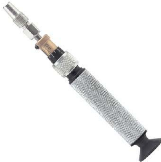
Figure 3.1 Utica TT-1 Torque Limiting Screwdriver used to apply small 2-4 in-oz torques to cap-screw assembly
