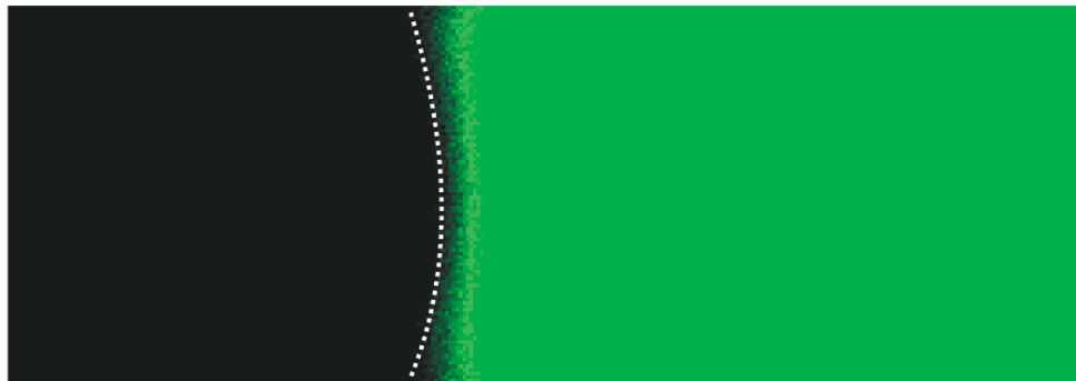
Figure 3.15: Confocal microscopy images of featureless channel cross-section at 2mm from inlet. Dashed line shows approximate diffusion boundary between the two fluids, demonstrating the “butterfly effect.”
