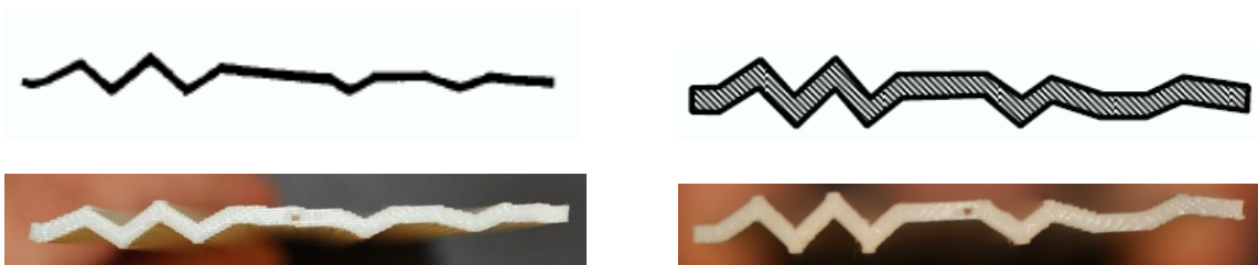
Figure 3-7: ABS Airfoil Comparison Kesel (2000) left, and Murphy (2009) right
