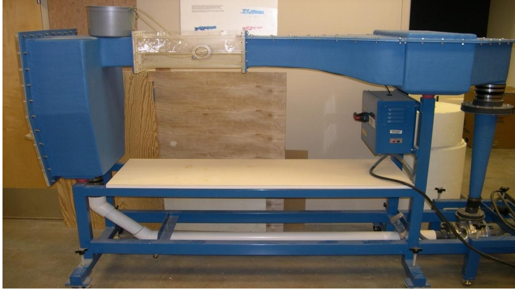
Figure 3-2: ELD Water Tunnel
