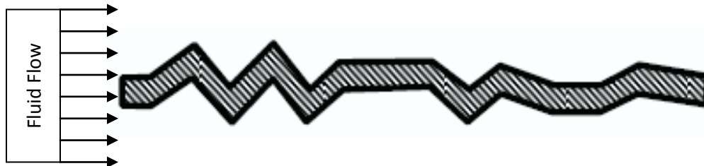
Figure 2-3: Murphy Corrugated Wing Cross Section (Murphy & Hu, 2009)
