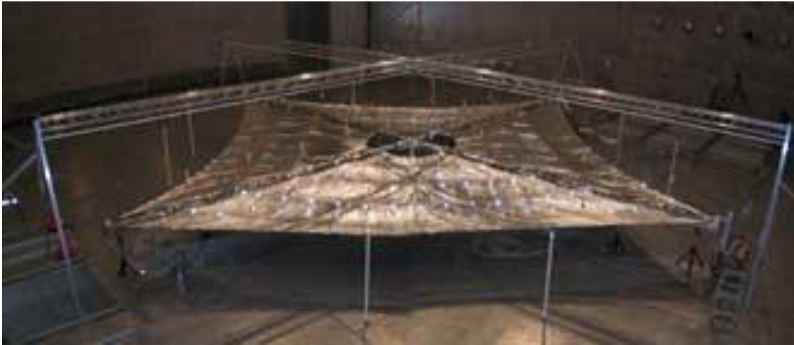
Figure 5: Solar Sail Measuring 33 ft. x 33 ft. (Jensen, 2004) (Image Courtesy of NASA)
