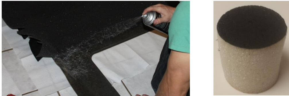
Figure 1.2 Sound absorbing materials with (a) adhesive (b) cover.
