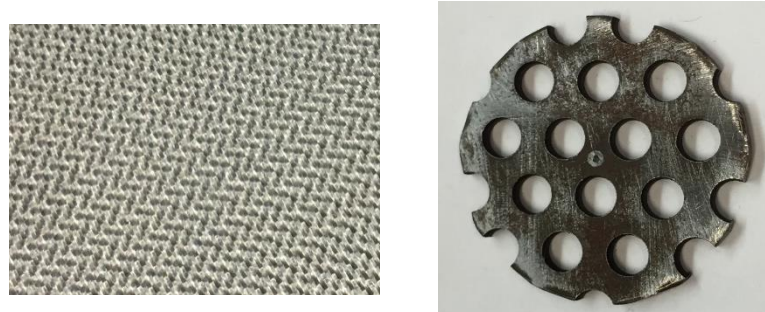
Figure 6.6 Photograph of a) Cover (armaglas fabrics) b) Perforated panel (steel)
