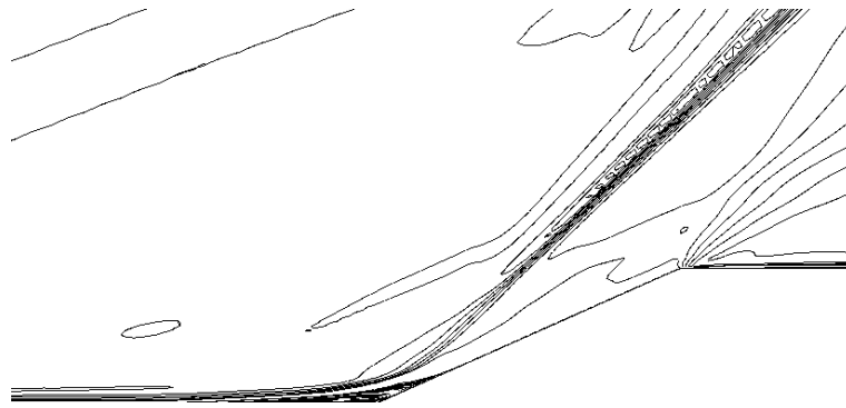
Figure 6.31: Contours of mean velocity for OVERFLOW's 5 th -order filtering with no turbulence model on an earlier mesh. Note the very long, thin separation zone and Gibbs phenomena upstream of the shock.
