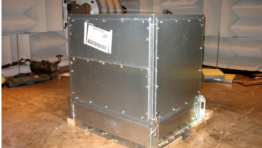
Figure 4.3 Air handler utilized for acoustic measurement
