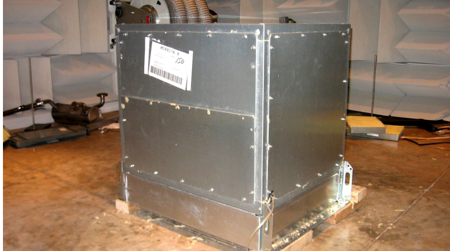
Figure 6.3 Air handler used for coupling loss factors measurement
