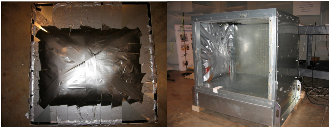
Figure 6.13 Panels heavily damped using sand bags
