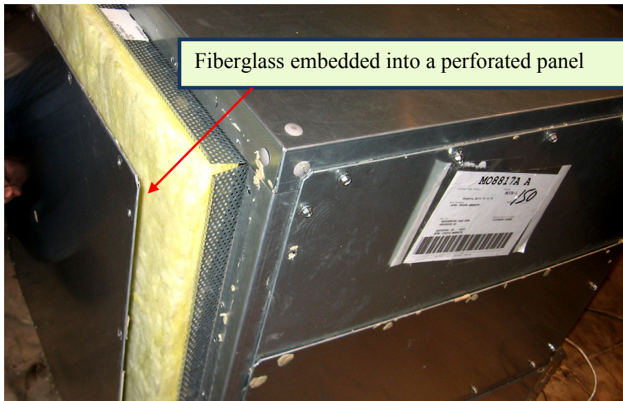
Figure 4.4 Fiberglass embedded into a perforated panel
