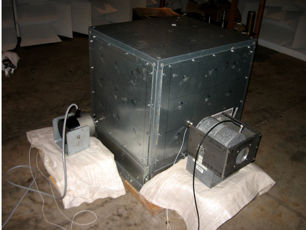
Figure 5.12 Air handler excited by two shakers
