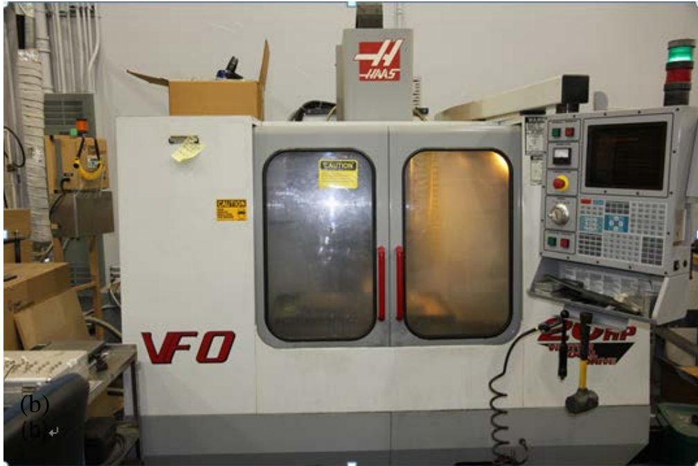
Figure 3.2: (a) Experimental setup of the drilling device; (b) HAAS VF-0 CNC vertical milling center.
