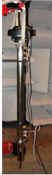
Figure 5.14 Vertical impedance tube measurement setup.
