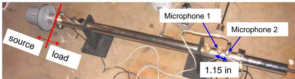
Figure 4.24 photograph showing measurement setup
