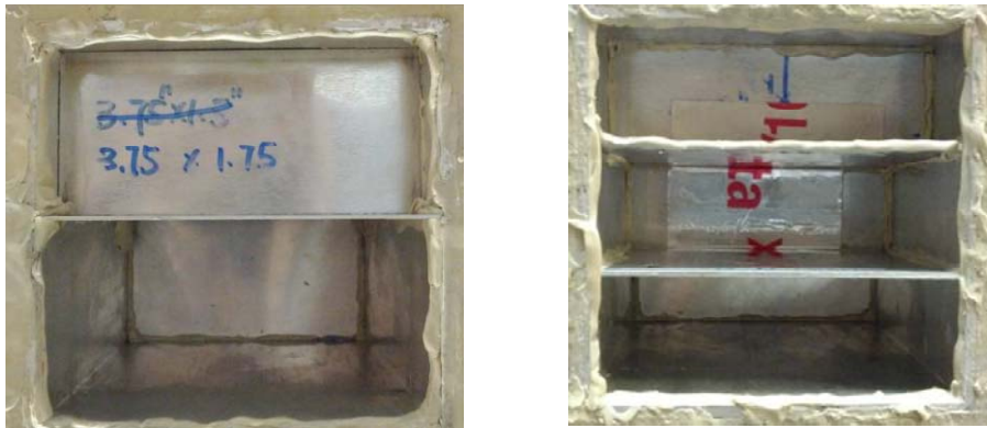
Figure 3.11 Photos of two-channel (left) and J-shape three-channel (right) backing design inside square impedance tube.
