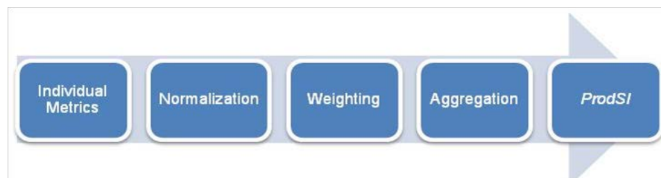
Figure 3-9 The five-step hierarchical ProdSI evaluation process
