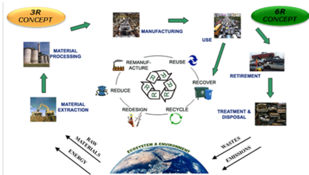
Figure 3-1 6R concept for a near perpetual material flow in a closed-loop
