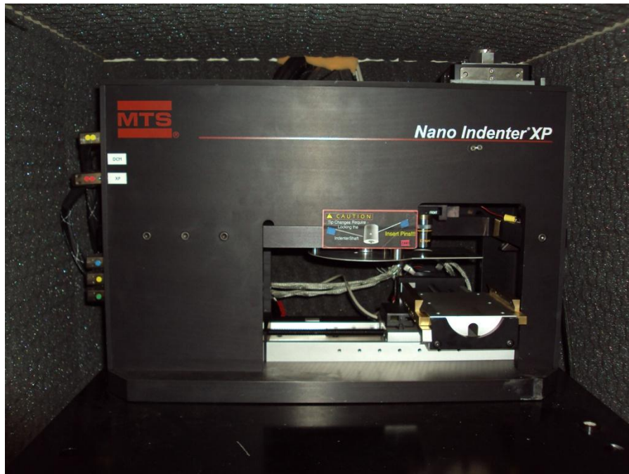
Figure 4.2. Photograph of the MTS Nano Indenter XP gantry and isolation cabinet.
