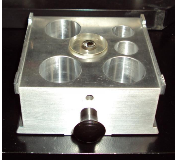
Figure 4.3. Image of aluminium testing stage used for modulus measurements.
