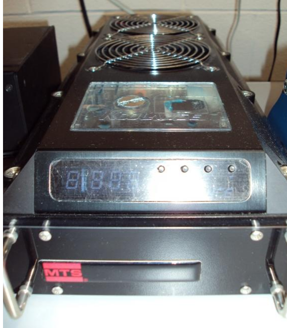
Figure 5.2. Coolant pump for the high temperature Nano Indenter XP.
