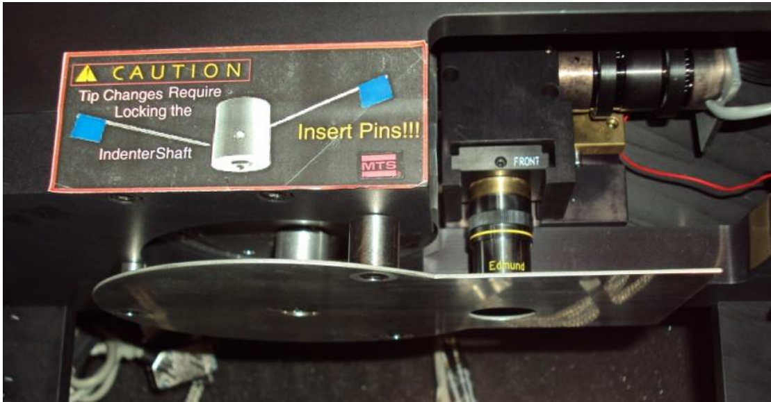
Figure 5.4. Heat shield installed on the MTS Nano Indenter XP.
