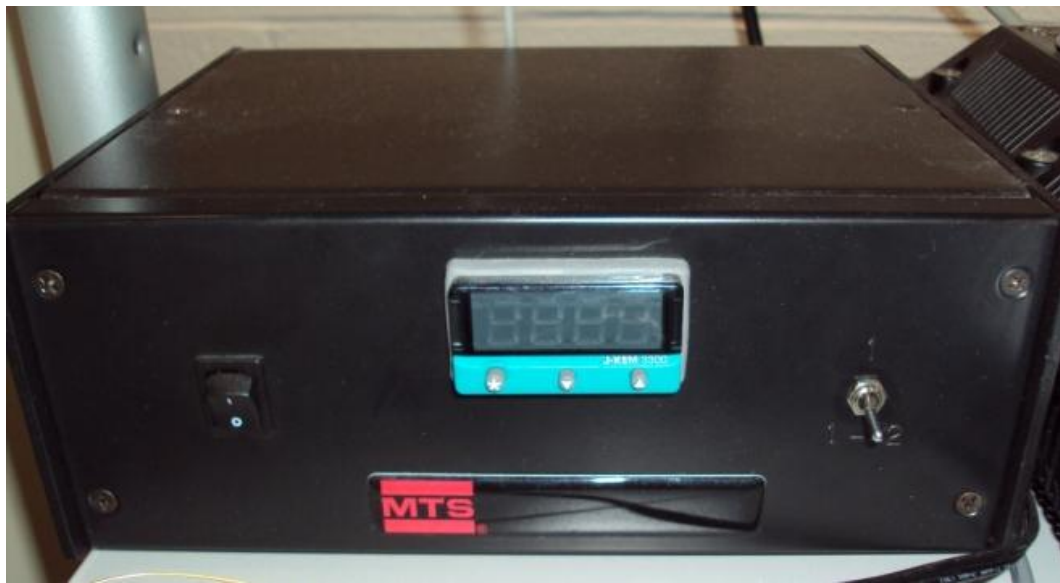
Figure 5.3. Variable DC output proportional controller for high temperature Nano Indenter XP.
