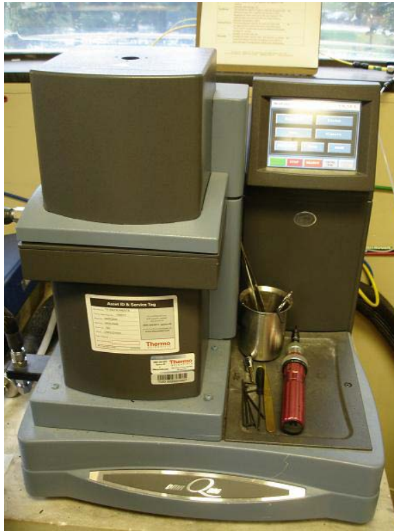
Figure 4-1: TA Instruments Q800 series DMA
