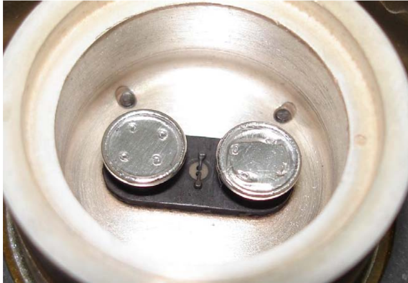
Figure 3-3: Sample pan and reference pan loaded in DSC
