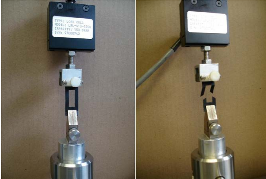
Figure 4-16: Left: Aperture card mounted to clamps; Right: Card cut, sample ready to test
