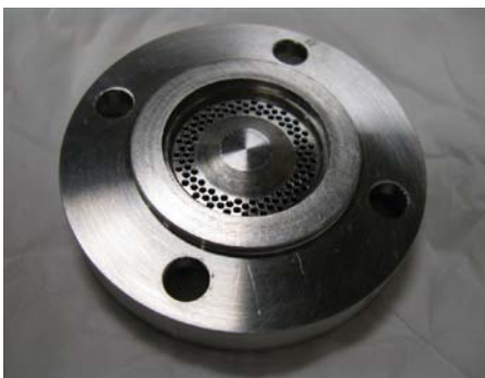
Figure 4.1. Dry-jet wet spinning die with 100 filament, 150 micron capillaries
