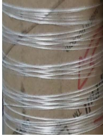
Figure 4.11. Low luster due to surface defects of wet-jet spun fiber
