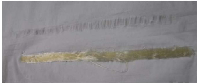
Figure 3.10. Excess solution removed from fiber using a Kimwipe
