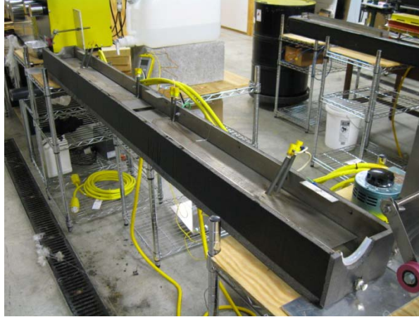
Figure 4.3. Hot steam stretch bath (shown without top in place)
