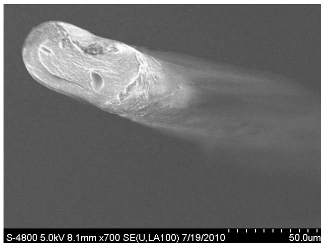
Figure 3.7. SEM image of skin-core structure of PAN precursor fiber produced at 30wt% DMAc/H 2 O and 35.8°C
