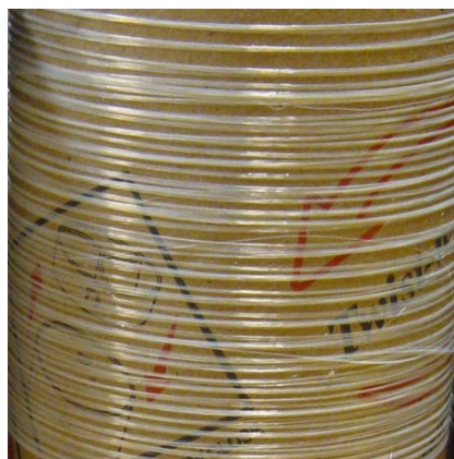
Figure 4.6. Dry-jet spun fiber stretched at 110 °C
