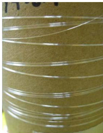
Figure 4.10. High luster of dry-jet spun fiber
