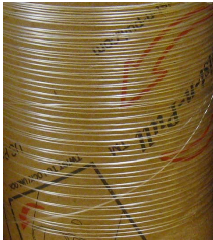
Figure 4.5. Wet-jet spun fiber stretched at 212 °C
