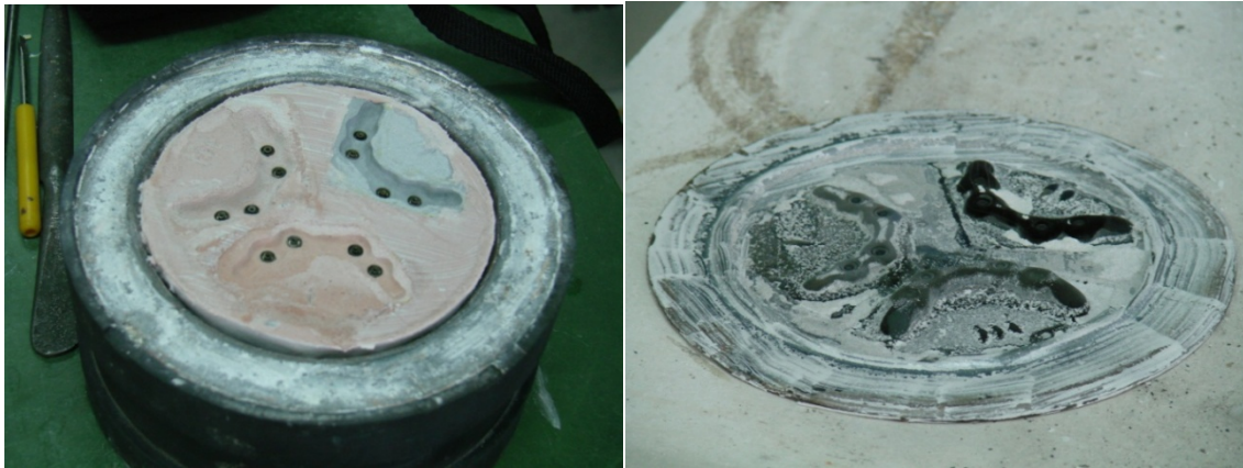
Figure 7: Mold inside steel chamber (Left); and formed titanium part (Right)
