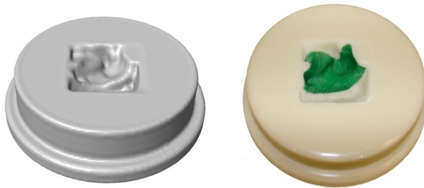
Figure 17: STL version of template (Left); rapid prototyped template (Right)
