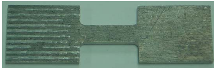
Figure 4.3: Slippage marks on a test specimen
