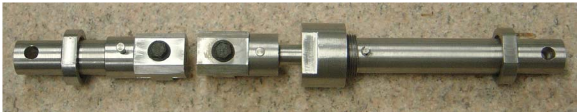
Figure 4.6: Type-I grips for high temperature tensile testing
