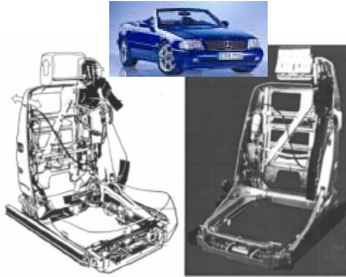
Figure 2.11: Magnesium seat frame for the SL-type, Mercedes Benz [Jambor and Beyer 1997]
