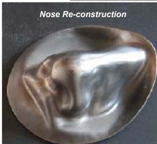
Figure 2.6: Superplastic forming used for medical applications [Curtis 2005]
