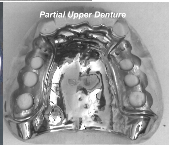
Figure 2.6: Superplastic forming used for medical applications [Curtis 2005]
