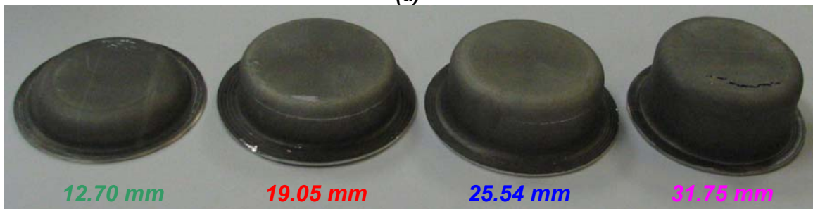
Figure 6.15: Pressure-time profiles for forming at 2 \times 10^{-4} \text{ s}^{-1} into multi-deep cylindrical dies (b) The corresponding formed parts
