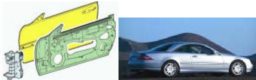
Figure 2.14: CL-type magnesium casting door inner part [Burk and Vogel 2002]
