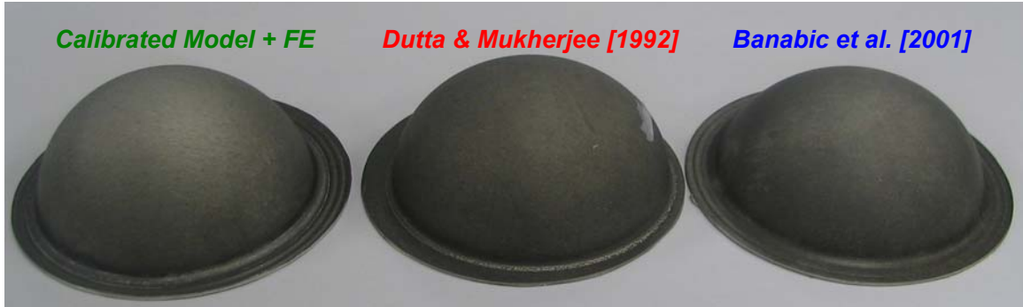
Figure 6.13: Formed domes using the three different forming pressure profiles
