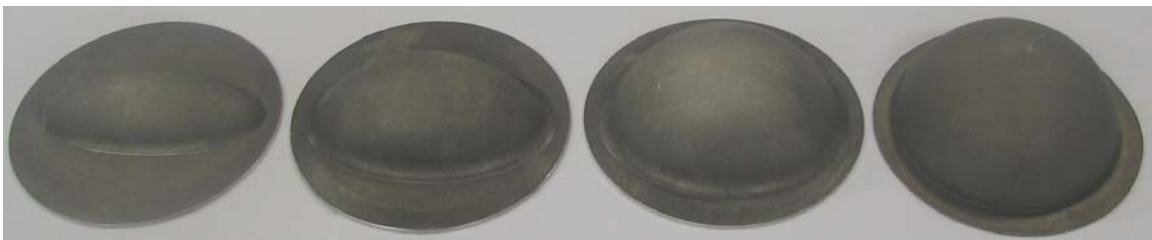
Figure 4.20: Examples for magnesium sheets formed into different shapes using type-II open elliptical forming dies
