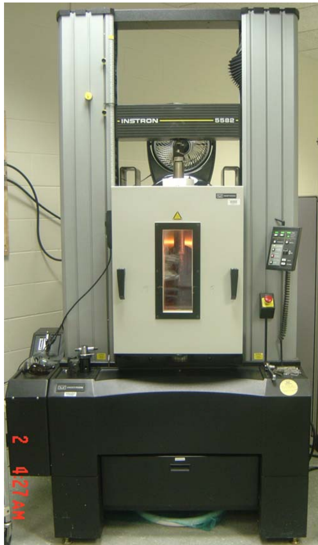
Figure 4.1: Load frame equipped with a heating chamber
