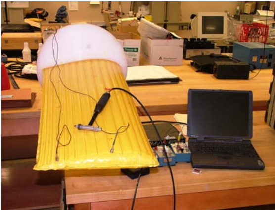
(a) Impact hammer test set-up.
