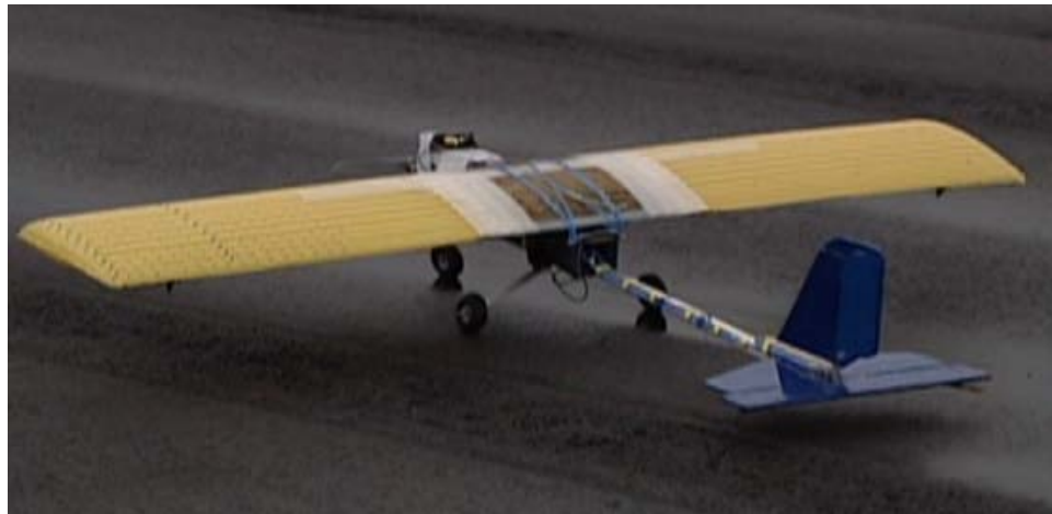
Figure 7.25: 2.44 m span Nylon wing flight test vehicle.
