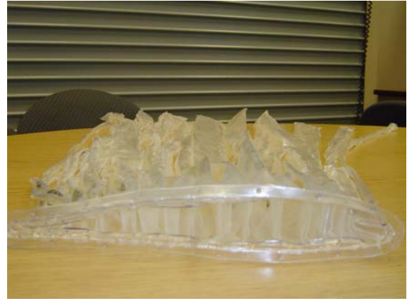
(b) Internal “finger-like” bladder.
