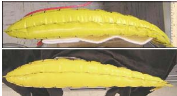
Figure 5.25: Inflatable wing with SMA chord morphing (deflected down and undeflected).
