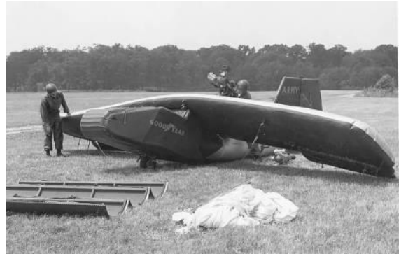
(b) Inflation and flight preparation of Inflatoplane
