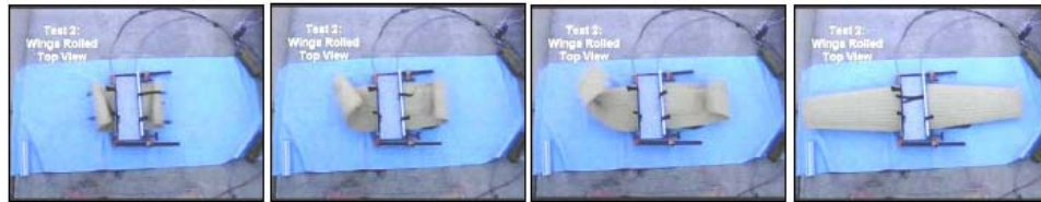
Figure 7.29: Rapid deployment testing of Vectran wing [32].
