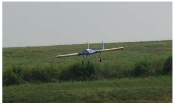
Figure 7.18: Flight test with Vectran wings on AIRCAT.
