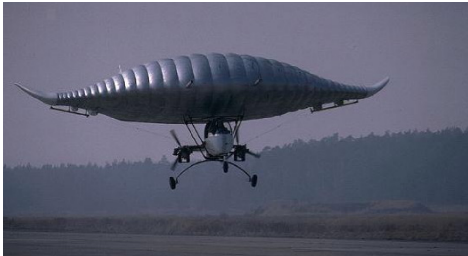
Figure 2.35: Prospective Concepts' "Stingray", a single seat inflatable wing aircraft [20].
