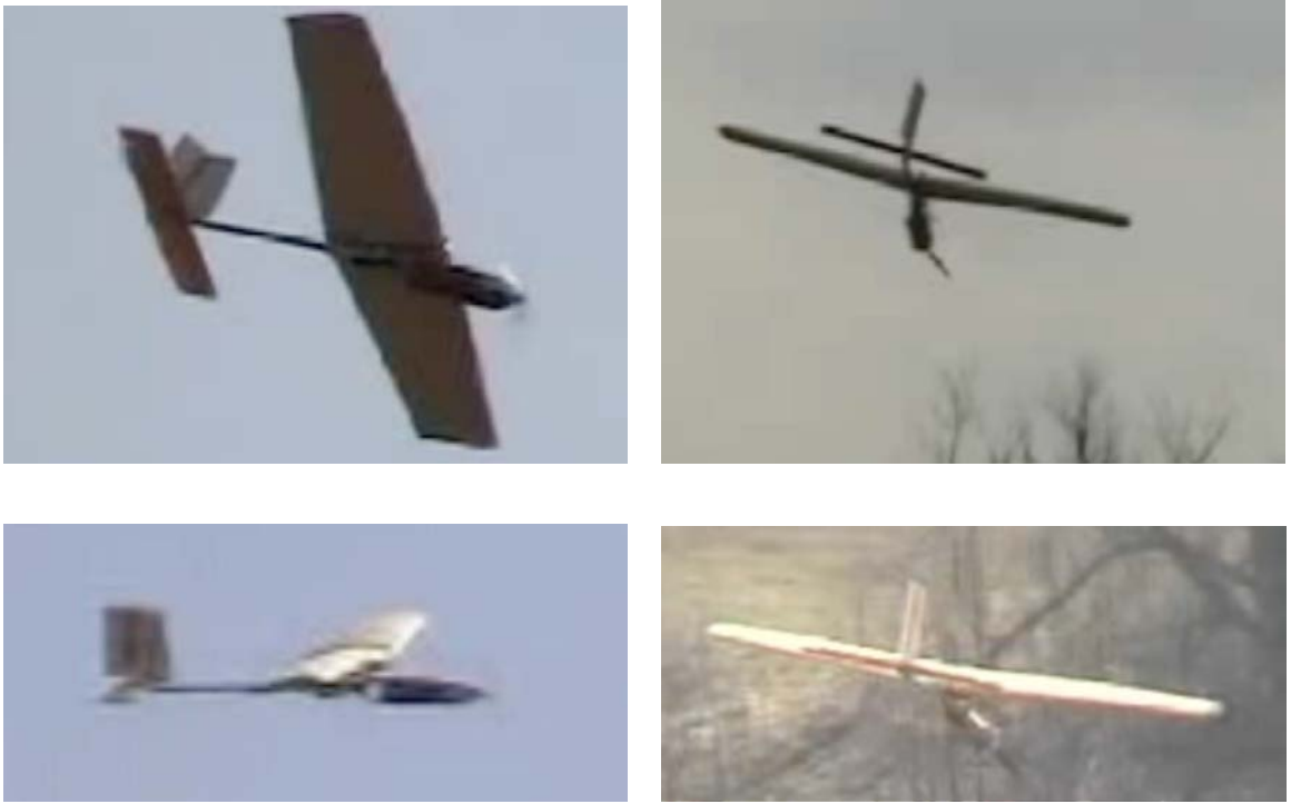
Figure 7.12: Flight test with wing warping of Vectran wings.
