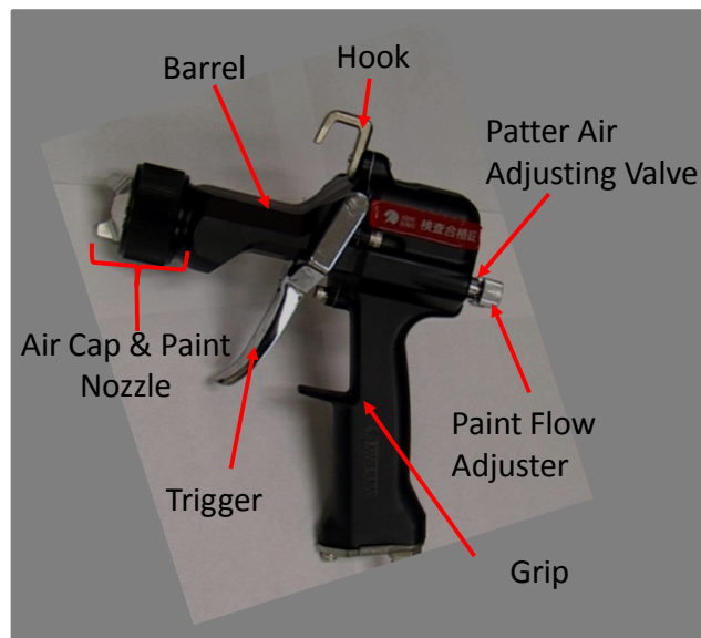
Figure 3.13: A picture of the HVLP air-assisted atomizer.
