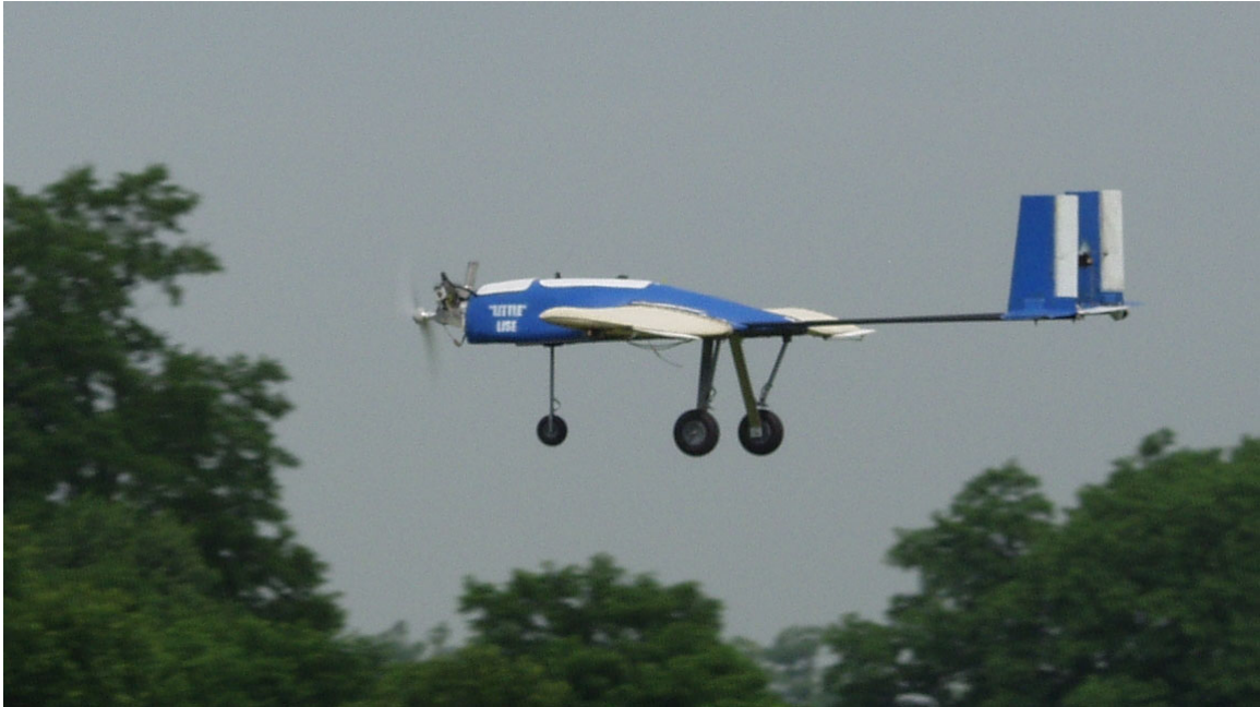
Figure 2.6 – Aircat UAV with inflatable wings
