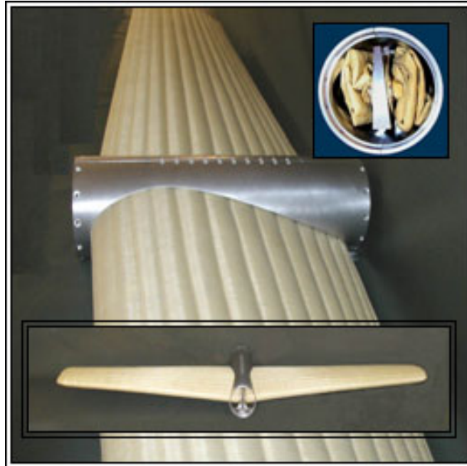
Figure 2.12 – Inflatable wings in packed and deployed configurations. (Image provided by ILC Dover)
