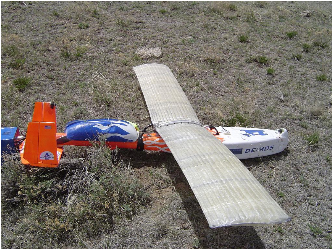
Figure 2.4 – BIG BLUE II glider after recovery with rigidized wings
