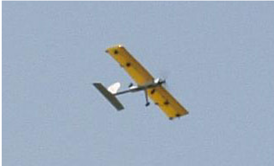
Figure 2.9 – In-flight photo of inflatable wing aircraft with servo actuated wing warping.
