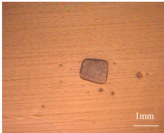
Fig. 5.6 Eutectic Sn-Pb over Polished Surface (vendor)
