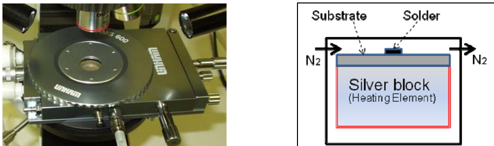
Fig. 4.3 Photo and schematic representation of Hot-stage chamber setup
