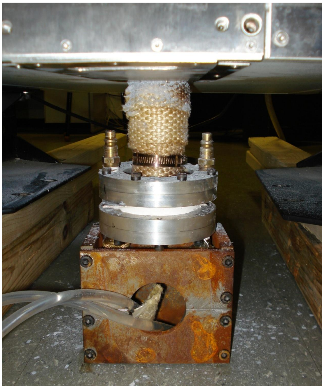
Figure 57 Picture of a different selective heating experiment using conduction from a furnace at 580°C this time with a 6061 T6 Aluminum heat source that is 1.5 inches in diameter
