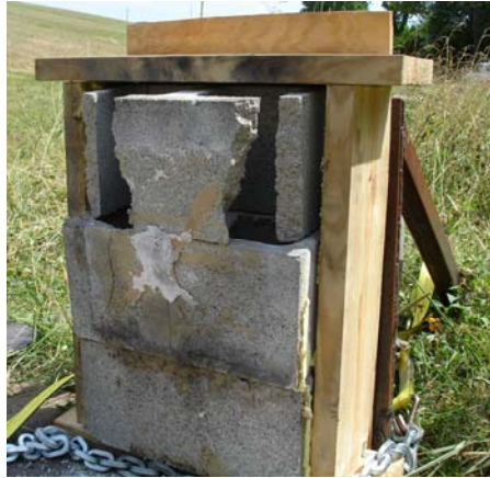
Figure 5.17 Result of Blast 1 – Drywall Only (Broken – Fail)
