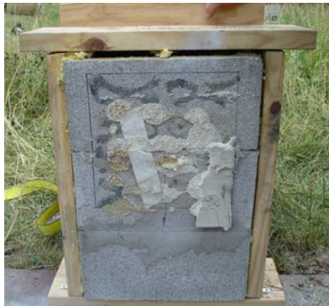
Figure 5.11 Result of Blast 5 – 4 lb. Ceno & 8 lb. Ceno & KFOAML1 (Intact – Pass)
