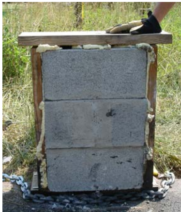
Figure 5.15 Result of Blast 9 – 4 lb. UFA & 8 lb. UFA & KFOAMLF (Intact – Pass)
