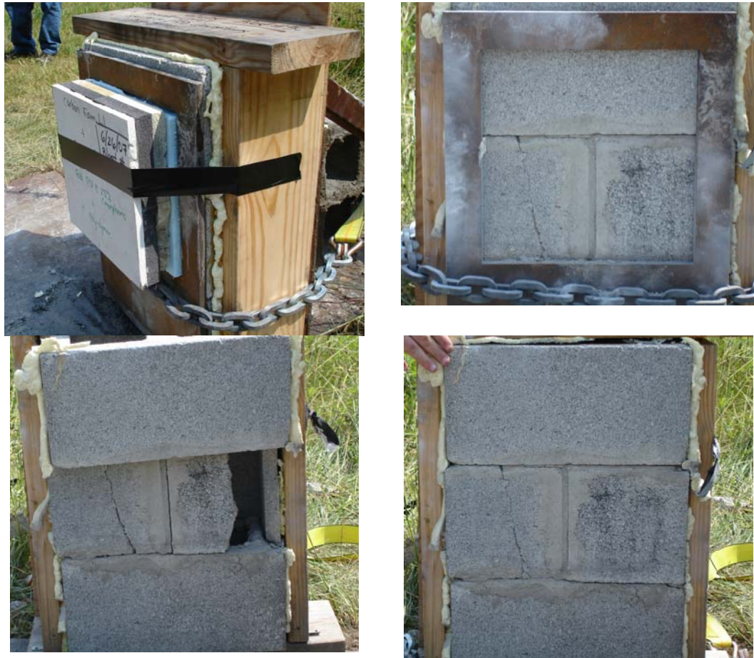
Figure C.11.a, b, c, d Blast 11 - Polystyrene & 8lb.Ceno & KFOAML1 (Clockwise from upper left) (a) Side view of front of foam sample before blast; (b) Front of mock wall after blast; (c) Front of mock wall after foam sample and steel plate were removed after blast; (d) Front of mock wall after blast after wall was tilted parallel with ground.
