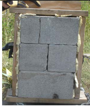
Figure C.15.a, b, c, d Blast 15 - 8lb. Ceno & KFOAML1 (Clockwise from upper left) (a) Front of foam sample before blast; (b) Front of mock wall immediately after blast; (c) Front of mock wall after tilting parallel with the ground after blast; (d) Front of mock wall immediately after blast.
