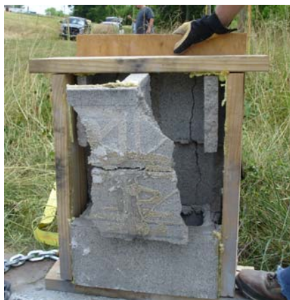
Figure 5.19 Result of Blast 3 – 2 Layers of Drywall and 16 Gage Steel (Broken – Fail)
