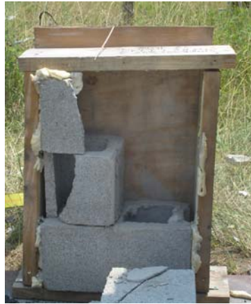
Figure 5.30 Result of Blast 14 – 8 lb. Ceno & KFOAML1 (Broken – Fail)
