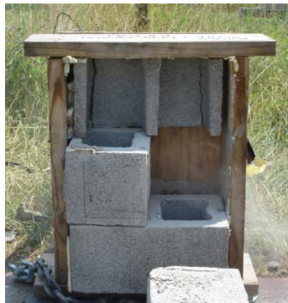
Figure 5.18 Result of Blast 12 – 4 lb. UFA & KFOAML1 (Broken – Fail)
