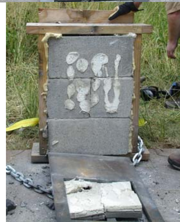
Figure C.8.a, b, c, d Blast 8 - 4lbCeno & 8lbUFA & KFOAML1 (Clockwise from upper left) (a) Front of foam sample before blast; (b) Front of foam sample after blast; (c) Front of mock wall after removing foam sample and steel plate. Some adhesive is visible; (d) Front of mock wall after blast.
