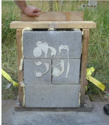
Figure 5.13 Result of Blast 7 – 4 lb. Ceno & 8lb. UFA & KFOAML (Intact – Pass)
