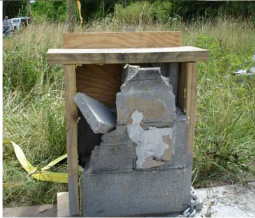
Figure C.2.a, b, c, d Blast 2 - Drywall & Drywall (Clock-wise from upper left) (a) Front of two layers of drywall before blast test; (b) Front of foam sample immediately after blast; (c) Condition of mock wall after removing foam sample and steel plate.
