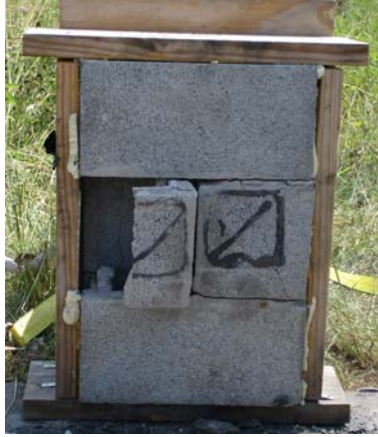
Figure 5.16 Result of Blast 10 – 4 lb. UFA & 8 lb. UFA & KFOAML1 (Broken – Fail)
