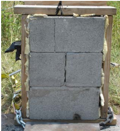
Figure C.15.a, b, c, d Blast 15 - 8lb. Ceno & KFOAML1 (Clockwise from upper left) (a) Front of foam sample before blast; (b) Front of mock wall immediately after blast; (c) Front of mock wall after tilting parallel with the ground after blast; (d) Front of mock wall immediately after blast.
