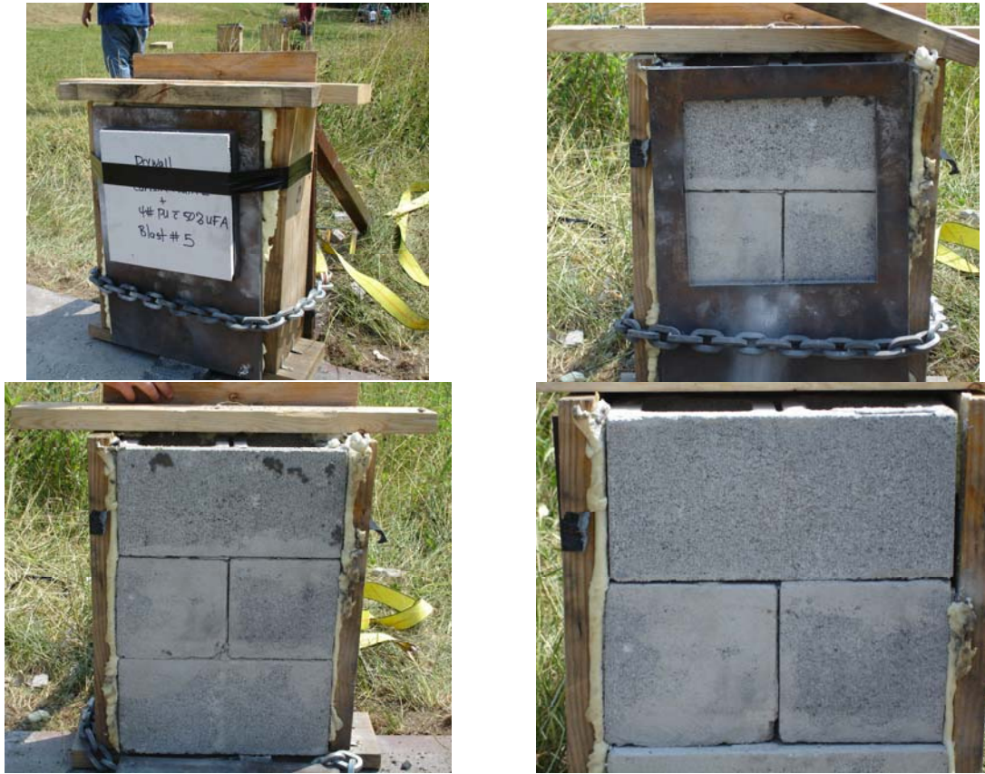
Figure C.13.a, b, c, d Blast 13 - 4lb.UFA & KFOAML (Clockwise from upper left) (a) Front of foam sample before blast; (b) Front of mock wall after blast; (c) Front of mock wall up close after foam sample and steel plate are removed after blast; (d) Front of mock wall after blast.
