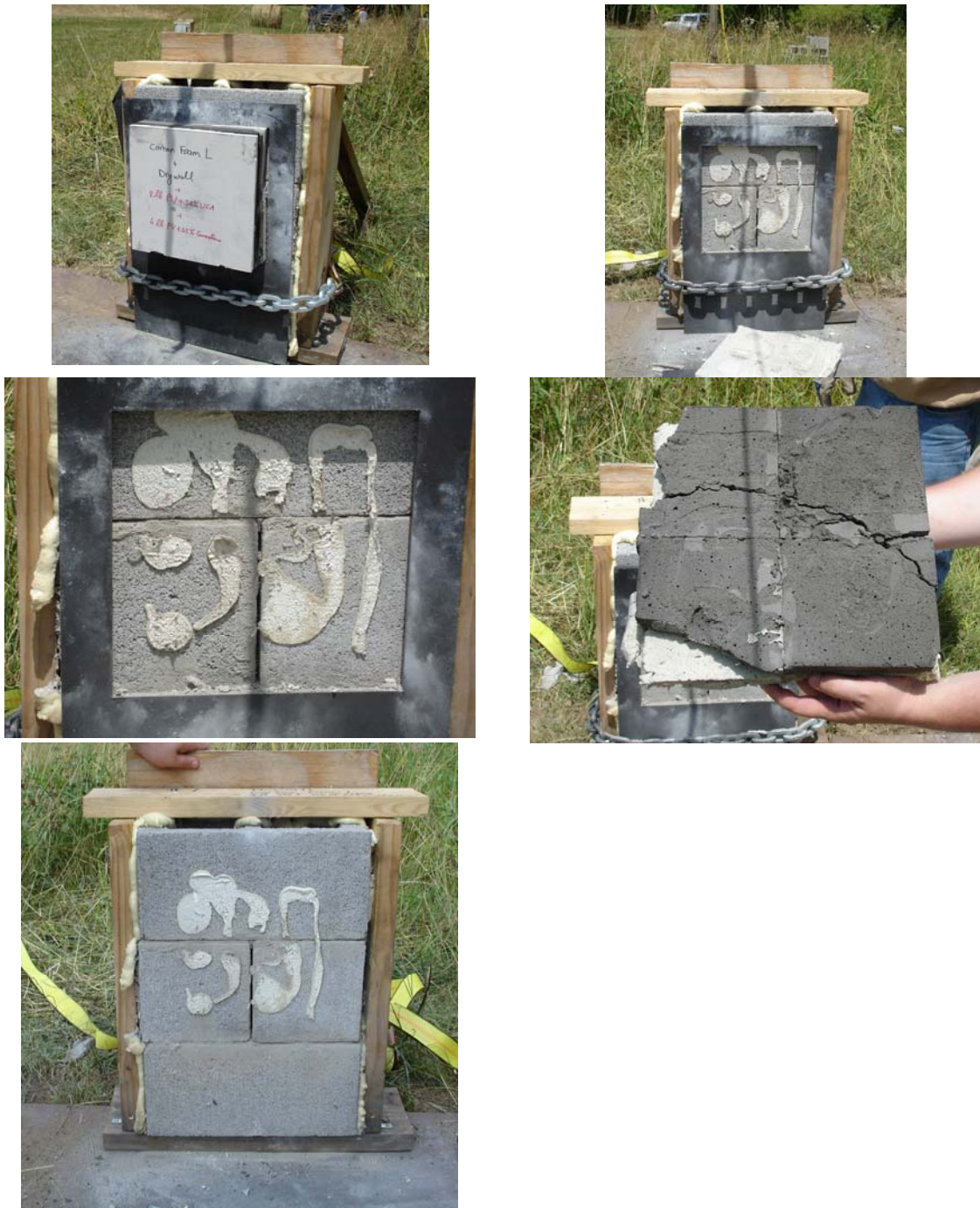
Figure C.7.a, b, c, d, e Blast 7 - 4lb.Ceno & 8lb.UFA & KFOAML (Clockwise from upper left) (a) Front of foam sample before blast; (b) Front of mock wall immediately after blast. Some adhesive is visible; (c) Condition of composite hybrid foam sample after blast; (d) Front of mock wall after removing foam sample and steel plate; (e) Up close view of mock wall area behind foam sample after blast.
