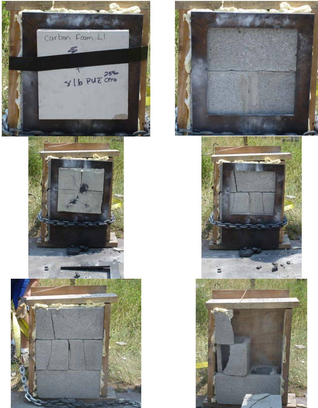
Figure C.14.a, b, c, d, e, f Blast 14 - 8lb.Ceno & KFOAML1 (Clockwise from upper left) (a) Front of foam sample before blast; (b) Front of mock wall before blast; (c) Front of mock wall after blast; (d) Mock wall after tilting parallel with ground after blast; (e) Front of mock wall immediately after blast; (f) Front of foam sample immediately after blast.
