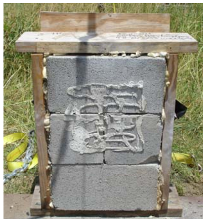
Figure 5.12 Result of Blast 6 – 4 lb. Ceno & 8 lb. Ceno & KFOAML (Intact – Pass)
