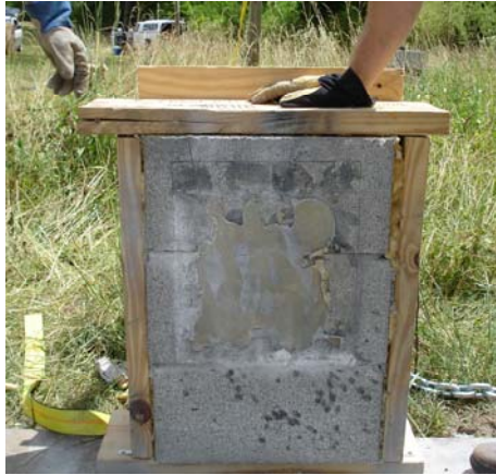
Figure 5.10 Result of Blast 4 – Polystyrene Foam, and 2 layers of Drywall (Cracked – Fail)
