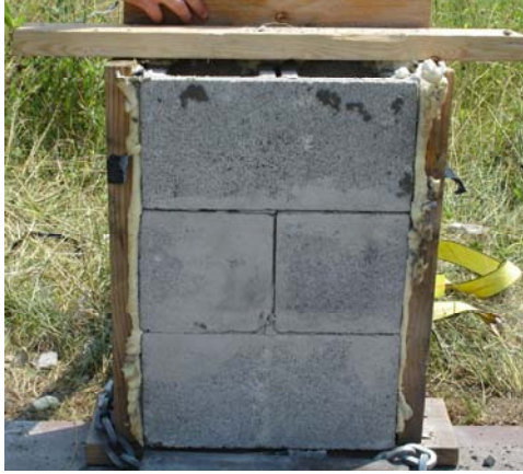
Figure 5.19 Result of Blast 13 – 4 lb. UFA & KFOAML (Cracked – Fail)
