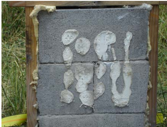
Figure 5.14 Result of Blast 8 – 4 lb. Ceno & 8 lb. UFA & KFOAML1 (Intact – Pass)
