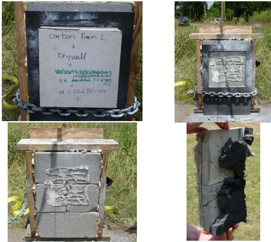
Figure C.6.a, b, c, d Blast 6 - 4lb.Ceno & 8lb.Ceno & KFOAML (Clockwise from upper left) (a) Front of foam sample before blast; (b) Front of mock wall immediately after blast. Some adhesive is visible; (c) Side view of foam sample remains after blast; (d) Front of mock wall after blast and after removing foam sample and steel plate.
