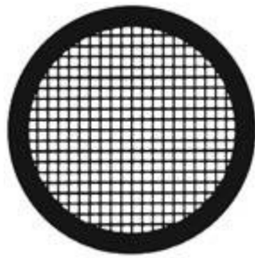
Figure 5.3: Transmission Electron Microscopy grids with 200 mesh, 3.05 mm O.D. Image source: https://www.tedpella.com/grids_html/maxtafrm.htm
