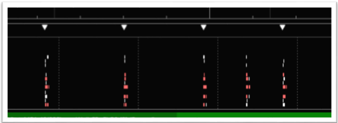
Figure 4.4: Example of ChR2 functional testing in rat cortical neuronal cultures. The screen displays waveforms detected in 16 electrodes in a single well of a 48 well plate. The blowup shows arrows which represent pulsed blue light. White and red dots indicate detected action potentials synchronized with the expression. Red dots in particular indicate neuron burst activity. Note that spontaneous firing activity also occurs without stimulus.
