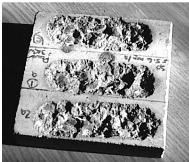
Figure 8.3. An example of the laser scabbling of concrete.
